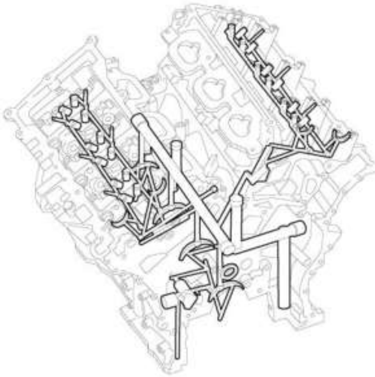
Fig. 516: Engine Lubrication Flow Courtesy of CHRYSLER GROUP, LLC
