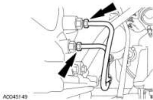
Fig. 251: Disconnecting Transmission Cooler Lines Courtesy of FORD MOTOR CO.
