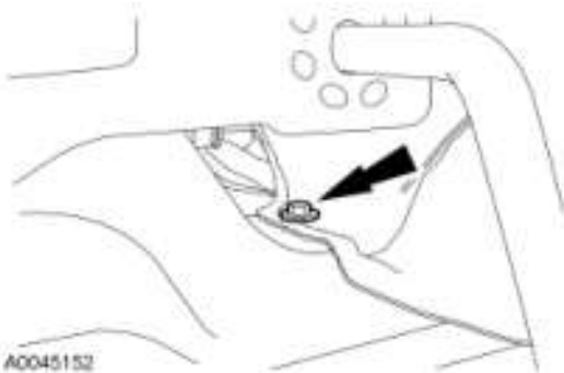
Fig. 254: Removing RH Exhaust Shield Bolt Courtesy of FORD MOTOR CO.
