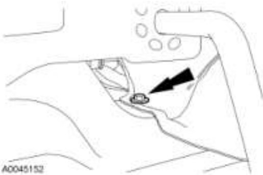
Fig. 230: Identifying RH Exhaust Shield Bolt Courtesy of FORD MOTOR CO.
