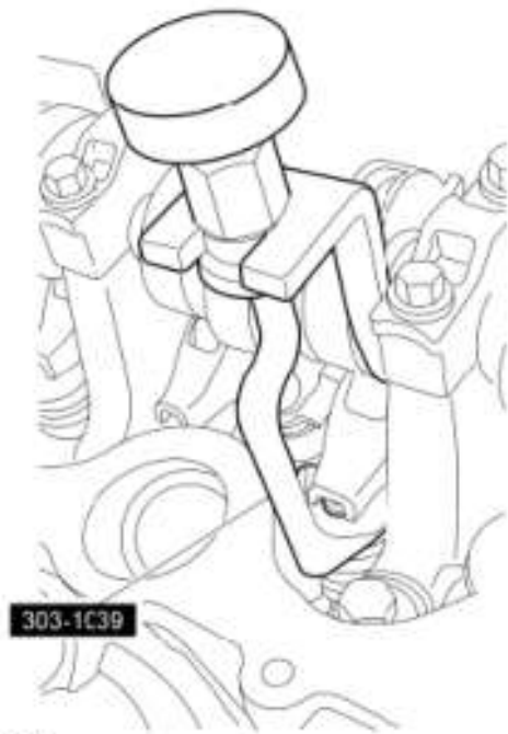
Fig. 335: Identifying Valve Spring Compressor (303-1039) Courtesy of FORD MOTOR CO.
