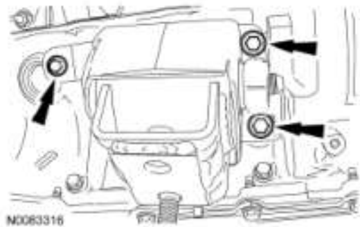
Fig. 312: Locating Bolts And RH Engine Support Insulator Courtesy of FORD MOTOR CO.
