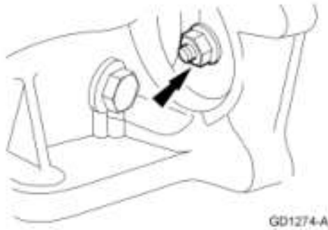
Fig. 280: Locating Torque Converter-To-Flexplate Nuts Courtesy of FORD MOTOR CO.
