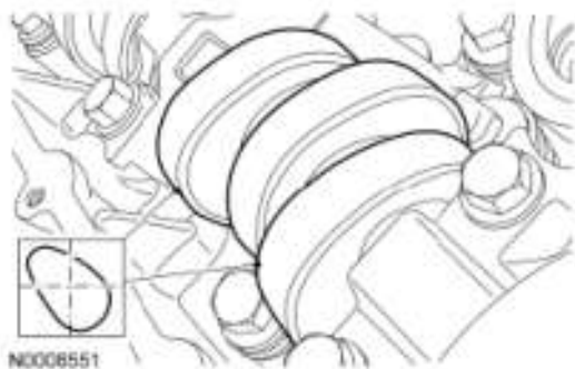
Fig. 331: Identifying Camshaft Lobes Courtesy of FORD MOTOR CO.
