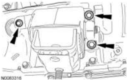
Fig. 314: Locating Engine Support Insulator Bolts Courtesy of FORD MOTOR CO.
