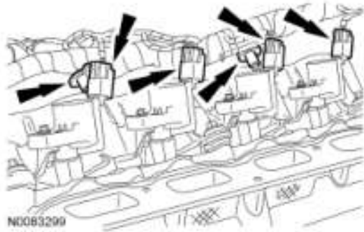
Fig. 303: Locating Ignition Coil Electrical Connectors And Engine Wiring Harness Retainers Courtesy of FORD MOTOR CO.
