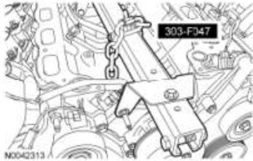
Fig. 311: Identifying Engine Lifting Bracket (303-F047) Courtesy of FORD MOTOR CO.
