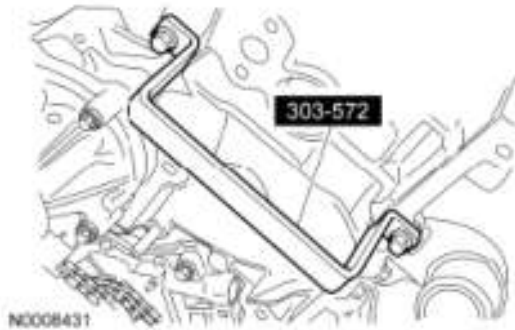
Fig. 344: Identifying Cylinder Head Remover/Installer (303-572) Courtesy of FORD MOTOR CO.
