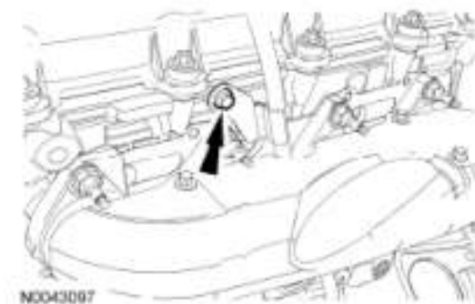
Fig. 320: Locating Oil Level Indicator Bolt Courtesy of FORD MOTOR CO.
