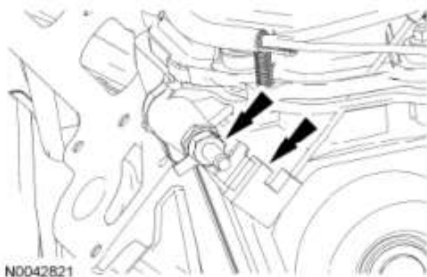
Fig. 318: Locating Nut And Radio Interference Capacitor Courtesy of FORD MOTOR CO.
