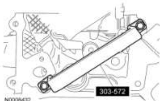
Fig. 355: Identifying Cylinder Head Remover/Installer (303-572) Courtesy of FORD MOTOR CO.
