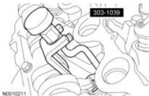
Fig. 333: Identifying Valve Spring Compressor (303-1039) Courtesy of FORD MOTOR CO.
