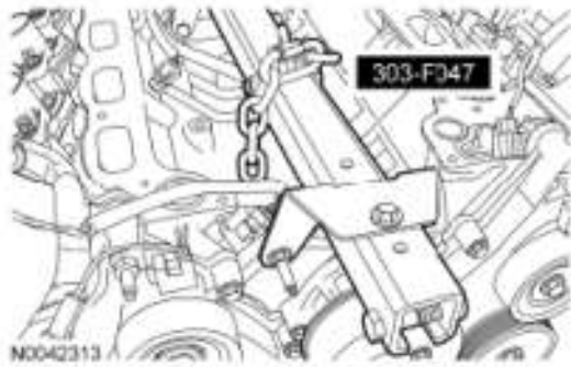
Fig. 364: Identifying Engine Lifting Bracket (303-F047) Courtesy of FORD MOTOR CO.
