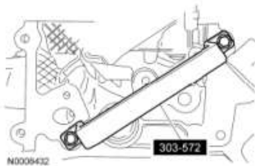
Fig. 410: Identifying Cylinder Head Remover/Installer (303-572) Courtesy of FORD MOTOR CO.
