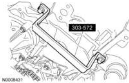
Fig. 409: Identifying Cylinder Head Remover/Installer (303-572) Courtesy of FORD MOTOR CO.
