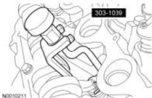
Fig. 399: Identifying Valve Spring Compressor (303-1039) Courtesy of FORD MOTOR CO.
