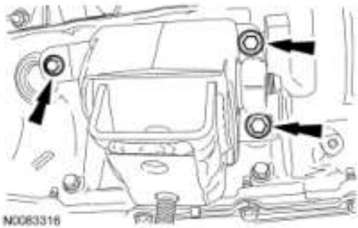
Fig. 365: Locating Engine Support Insulator Bolts Courtesy of FORD MOTOR CO.
