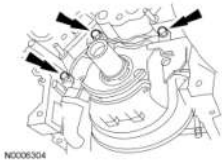
Fig. 418: Locating Oil Pump And Bolts Courtesy of FORD MOTOR CO.
