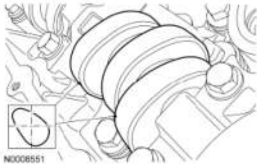
Fig. 397: Identifying Camshaft Lobes Courtesy of FORD MOTOR CO.
