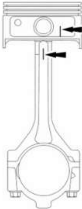
Fig. 433: Locating Mark On Piston And Connecting Rod Courtesy of FORD MOTOR CO.
