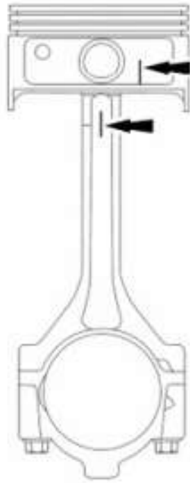
Fig. 434: Locating Mark On Piston And Connecting Rod Courtesy of FORD MOTOR CO.
