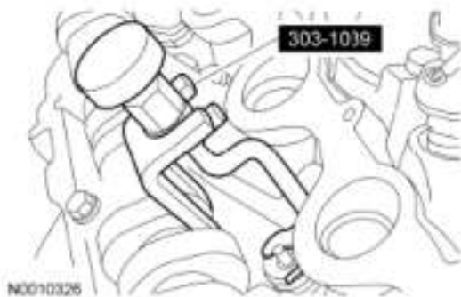
Fig. 429: Identifying Valve Spring Compressor (303-1039) Courtesy of FORD MOTOR CO.
