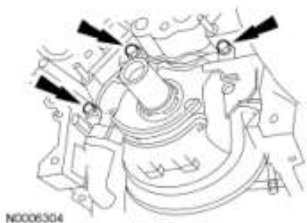
Fig. 449: Locating Oil Pump And Bolts Courtesy of FORD MOTOR CO.
