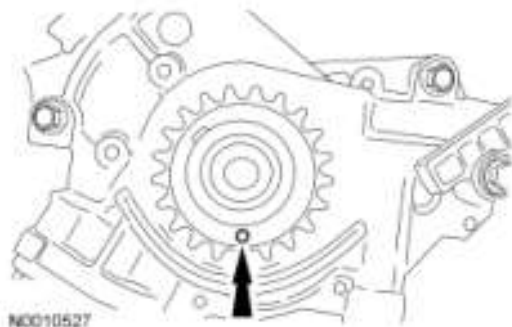
Fig. 462: Locating Crankshaft Sprocket Timing Mark Courtesy of FORD MOTOR CO.
