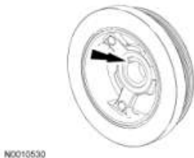
Fig. 484: Locating Woodruff Key Slot Courtesy of FORD MOTOR CO.
