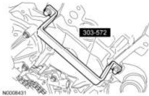
Fig. 455: Identifying Cylinder Head Remover/Installer (303-572) Courtesy of FORD MOTOR CO.
