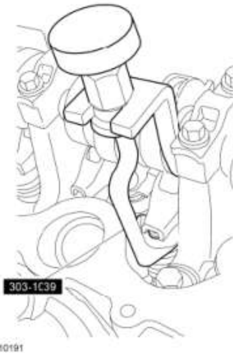
Fig. 478: Identifying Valve Spring Compressor (303-1039) Courtesy of FORD MOTOR CO.
