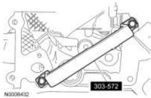
Fig. 456: Identifying Cylinder Head Remover/Installer (303-572) Courtesy of FORD MOTOR CO.
