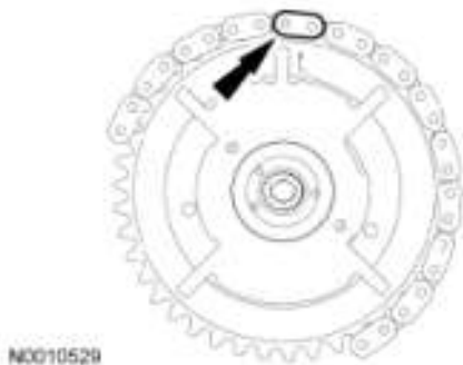
Fig. 469: Locating Camshaft Sprocket Timing Mark With Copper Link Courtesy of FORD MOTOR CO.
