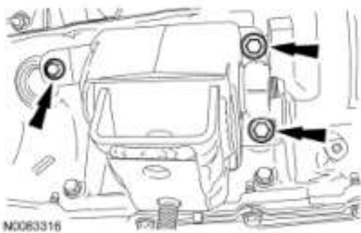
Fig. 496: Locating Engine Support Insulator Bolts Courtesy of FORD MOTOR CO.
