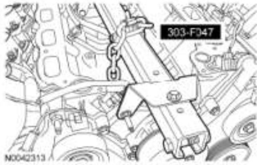
Fig. 512: Identifying Engine Lifting Bracket (303-F047) Courtesy of FORD MOTOR CO.
