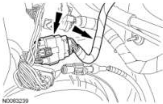
Fig. 546: Locating Wiring Harness And Electrical Connector Retainers Courtesy of FORD MOTOR CO.
