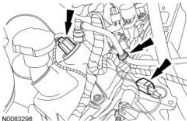
Fig. 541: Locating Variable Camshaft Timing (VCT) Solenoid And Radio Ignition Interference Capacitor Electrical Connectors
