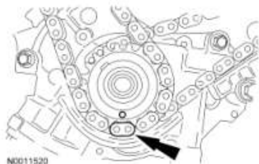
Fig. 588: Aligning Timing Mark On Sprocket With Single Colored (Marked) Chain Link Courtesy of FORD MOTOR CO.
