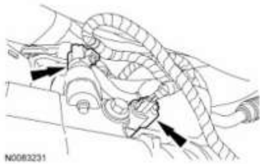
Fig. 548: Locating A/C Compressor Electrical Connector And Wiring Harness Retainer Courtesy of FORD MOTOR CO.
