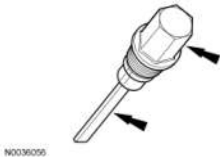
Fig. 33: Locating Fluid Level Indicator And Fill Plug Courtesy of FORD MOTOR CO.
