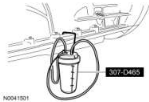
Fig. 23: Hanging Special Tool (307-D465) Under Vehicle, Upright & Close To Transmission Courtesy of FORD MOTOR CO.
