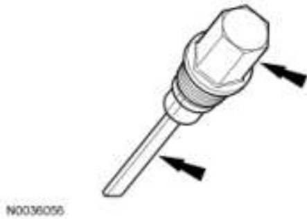
Fig. 17: Locating Fluid Level Indicator And Fill Plug Courtesy of FORD MOTOR CO.
