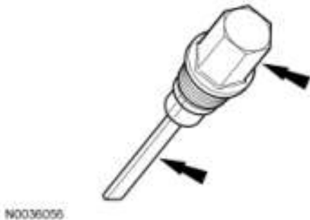
Fig. 12: Locating Fluid Level Indicator And Fill Plug Courtesy of FORD MOTOR CO.
