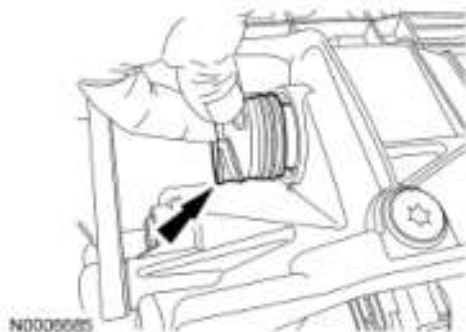
Fig. 55: Locating Outer Shell Of Bulkhead Electrical Connector Courtesy of FORD MOTOR CO.
