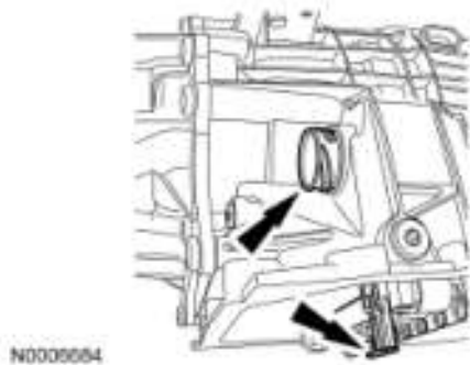
Fig. 54: Locating Outer Shell Of Bulkhead Electrical Connector Courtesy of FORD MOTOR CO.
