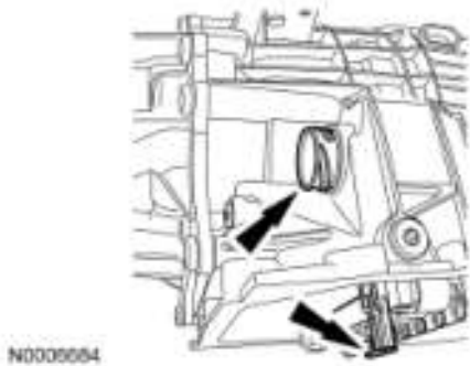
Fig. 101: Locating Outer Shell Of Bulkhead Electrical Connector Courtesy of FORD MOTOR CO.
