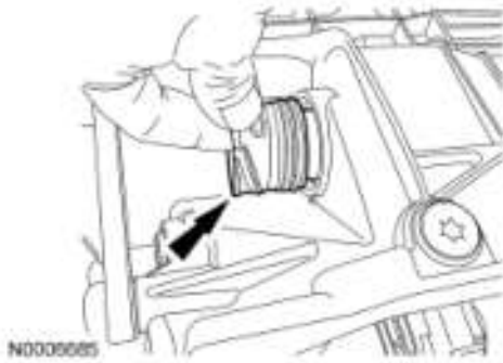
Fig. 87: Locating Outer Shell Of Bulkhead Electrical Connector Courtesy of FORD MOTOR CO.
