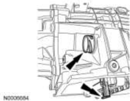
Fig. 86: Locating Outer Shell Of Bulkhead Electrical Connector Courtesy of FORD MOTOR CO.
