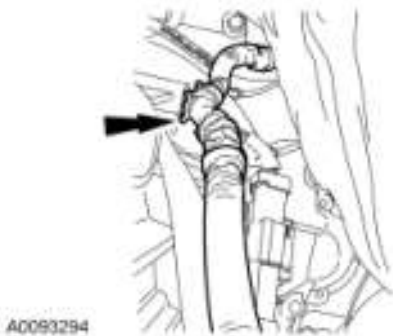
Fig. 130: Locating Wire Harness From Top Of Transmission Courtesy of FORD MOTOR CO.
