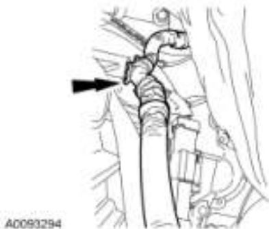
Fig. 158: Locating Wire Harness From Top Of Transmission Courtesy of FORD MOTOR CO.
