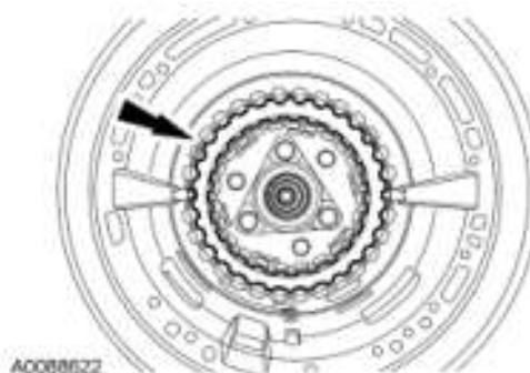
Fig. 185: Locating Low/Reverse Clutch Pack Courtesy of FORD MOTOR CO.
