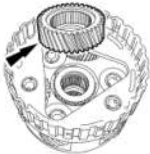
Fig. 187: Locating Low/Reverse Sun Gear Courtesy of FORD MOTOR CO.
