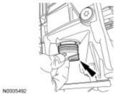
Fig. 169: Locating Outer Shell Of Bulkhead Electrical Connector Courtesy of FORD MOTOR CO.
