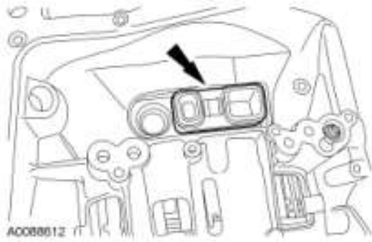
Fig. 172: Locating Rubber Adapter Courtesy of FORD MOTOR CO.
