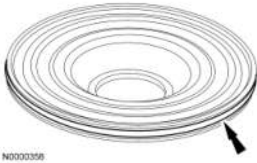
Fig. 260: Overdrive Clutch Balance Piston O-Ring Seal Courtesy of FORD MOTOR CO.
