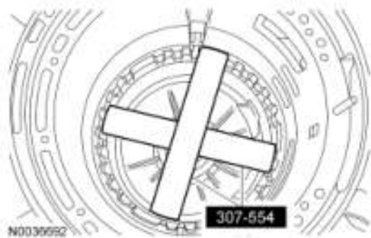
Fig. 337: Installing Special Tool (307-554) Into Case Courtesy of FORD MOTOR CO.
