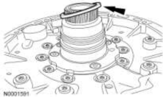
Fig. 368: Locating Front Pump Washer Courtesy of FORD MOTOR CO.
