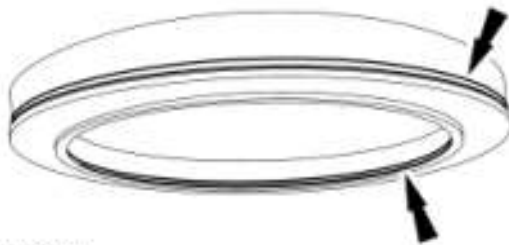
Fig. 313: Locating Inner And Outer Intermediate Clutch Piston O-Ring Seals Courtesy of FORD MOTOR CO.
