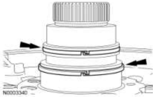
Fig. 358: Locating Front Pump Seal Rings Courtesy of FORD MOTOR CO.
