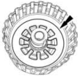
Fig. 263: Locating Overdrive Clutch Return Spring Courtesy of FORD MOTOR CO.
