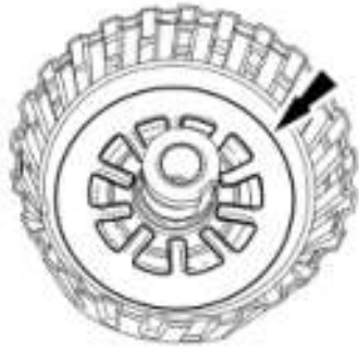
Fig. 254: Locating Overdrive Clutch Return Spring Courtesy of FORD MOTOR CO.
