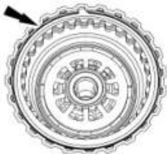
Fig. 301: Locating Direct Clutch Snap Ring Courtesy of FORD MOTOR CO.
