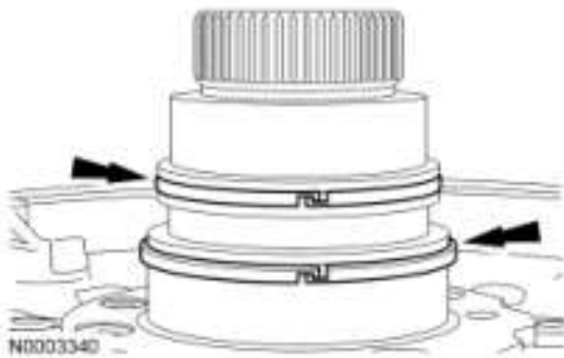
Fig. 365: Locating Front Pump Seal Rings Courtesy of FORD MOTOR CO.
