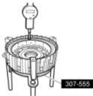
Fig. 246: Installing Forward Clutch Assembly Into Special Tool (307-555) Courtesy of FORD MOTOR CO.
