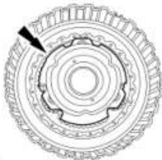
Fig. 247: Locating Sun Gear Into Forward Clutch Drum Courtesy of FORD MOTOR CO.
