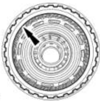
Fig. 308: Locating Intermediate Clutch Plates Courtesy of FORD MOTOR CO.
