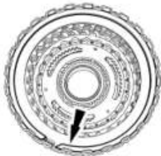
Fig. 245: Locating Forward Clutch Pack Snap Ring Courtesy of FORD MOTOR CO.
