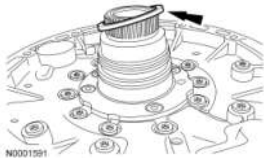
Fig. 356: Locating Front Pump Washer Courtesy of FORD MOTOR CO.
