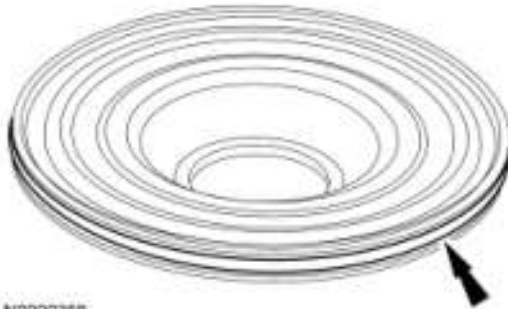
Fig. 256: Overdrive Clutch Balance Piston O-Ring Seal Courtesy of FORD MOTOR CO.
