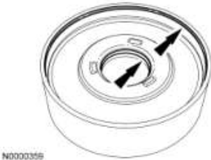
Fig. 261: Locating O-Ring Seals On Overdrive Clutch Apply Piston Courtesy of FORD MOTOR CO.
