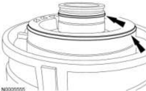
Fig. 331: Locating Low/Reverse Drum O-Ring Seals Courtesy of FORD MOTOR CO.
