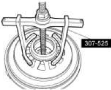
Fig. 334: Installing Retaining Ring Using Special Tool (307-525) Courtesy of FORD MOTOR CO.
