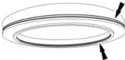
Fig. 314: Locating Inner And Outer Intermediate Clutch Piston O-Ring Seals Courtesy of FORD MOTOR CO.
