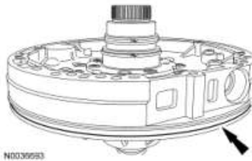
Fig. 366: Locating Pump Outer Diameter Front Pump O-Ring Seal Courtesy of FORD MOTOR CO.
