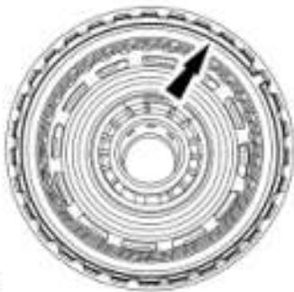
Fig. 307: Locating Intermediate Clutch Plate Snap Ring Courtesy of FORD MOTOR CO.
