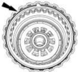
Fig. 279: Locating Direct Clutch Snap Ring Courtesy of FORD MOTOR CO.
