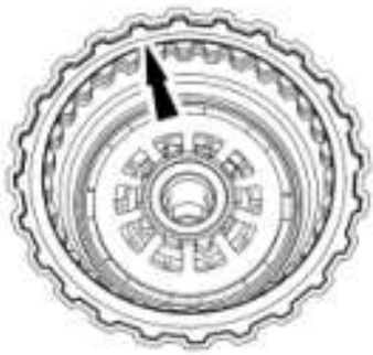
Fig. 280: Locating Direct Clutch Steel And Friction Plates Courtesy of FORD MOTOR CO.
