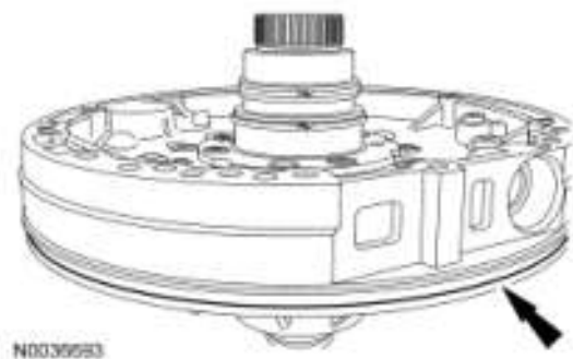
Fig. 357: Locating Pump Outer Diameter Front Pump O-Ring Seal Courtesy of FORD MOTOR CO.
