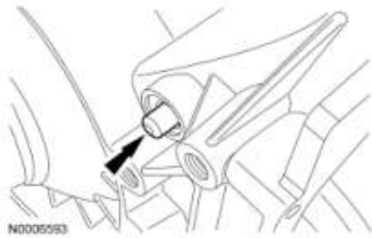
Fig. 381: Positioning Park Pawl Pin Into Case Courtesy of FORD MOTOR CO.
