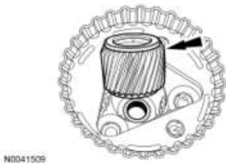
Fig. 394: Locating Sun Gear Into Planet Assembly Courtesy of FORD MOTOR CO.
