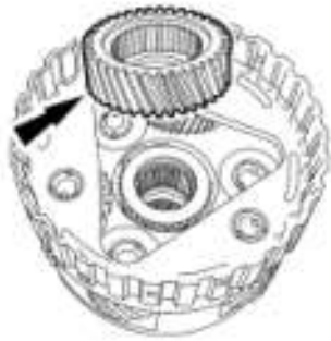
Fig. 395: Locating Low/Reverse Sun Gear Courtesy of FORD MOTOR CO.
