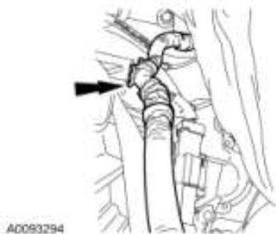
Fig. 435: Locating Wire Harness From Top Of Transmission Courtesy of FORD MOTOR CO.
