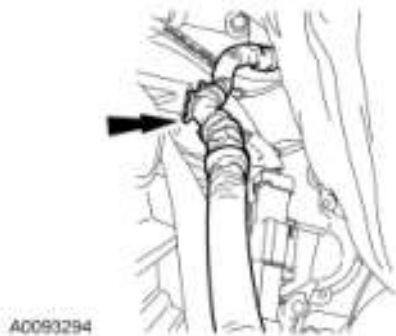
Fig. 462: Locating Wire Harness From Top Of Transmission Courtesy of FORD MOTOR CO.
