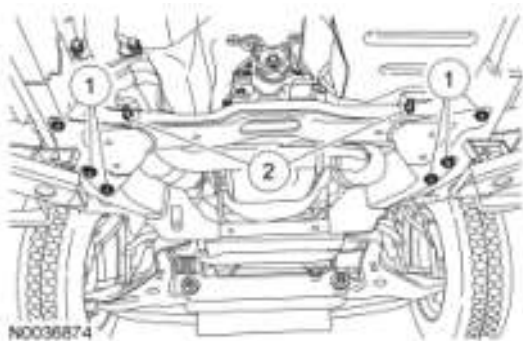
Fig. 469: Identifying Crossmember Bolts Courtesy of FORD MOTOR CO.
