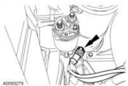
Fig. 478: Locating Ground Wire Stud Courtesy of FORD MOTOR CO.
