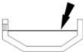
Fig. 1: Identifying Transfer Case Oil Level Courtesy of FORD MOTOR CO.
