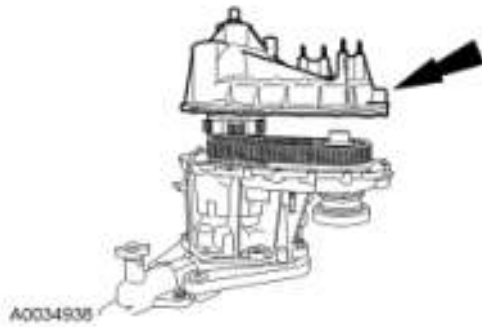
Fig. 159: Assembling Front And Rear Case Halves Courtesy of FORD MOTOR CO.
