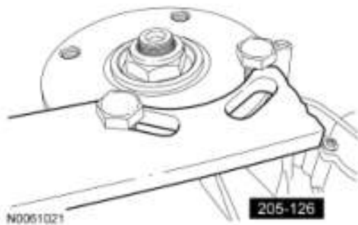
Fig. 98: Removing Nut Using Special Tool (205-126) To Hold Output Flange Courtesy of FORD MOTOR CO.
