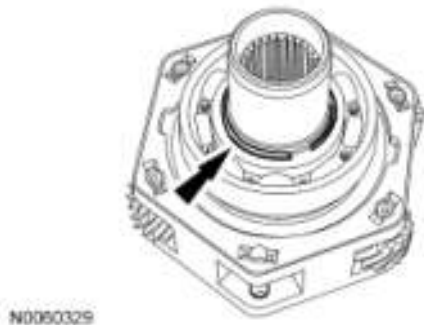
Fig. 140: Locating Snap Ring Courtesy of FORD MOTOR CO.
