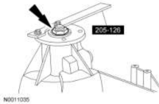
Fig. 53: Locating Output Flange Nut And Special Tool (205-126) Courtesy of FORD MOTOR CO.
