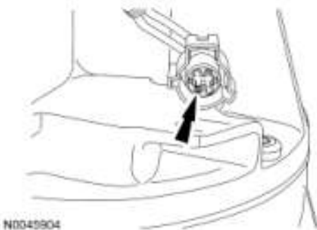
Fig. 56: Locating Coil Wire Electrical Connector Courtesy of FORD MOTOR CO.
