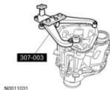
Fig. 95: Securing Transfer Case To Bench Courtesy of FORD MOTOR CO.
