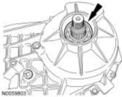
Fig. 21: Locating Bearing Courtesy of FORD MOTOR CO.
