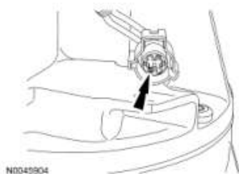
Fig. 93: Locating Coil Wire Electrical Connector Courtesy of FORD MOTOR CO.
