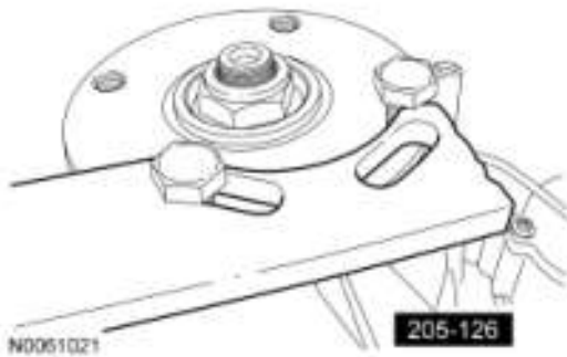
Fig. 162: Installing Nut Using Special Tool (205-126) To Hold Output Flange Courtesy of FORD MOTOR CO.
