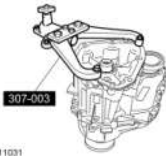
Fig. 51: Securing Transfer Case To Bench Courtesy of FORD MOTOR CO.
