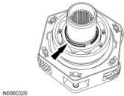
Fig. 125: Locating Snap Ring Courtesy of FORD MOTOR CO.
