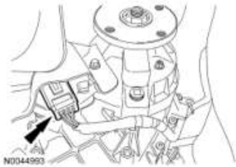
Fig. 176: Locating Shift Motor Electrical Connector Courtesy of FORD MOTOR CO.
