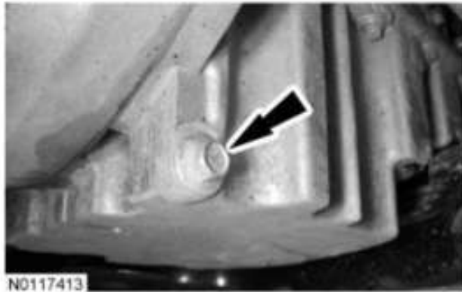
Fig. 475: Locating Drain Plug Courtesy of FORD MOTOR CO.
