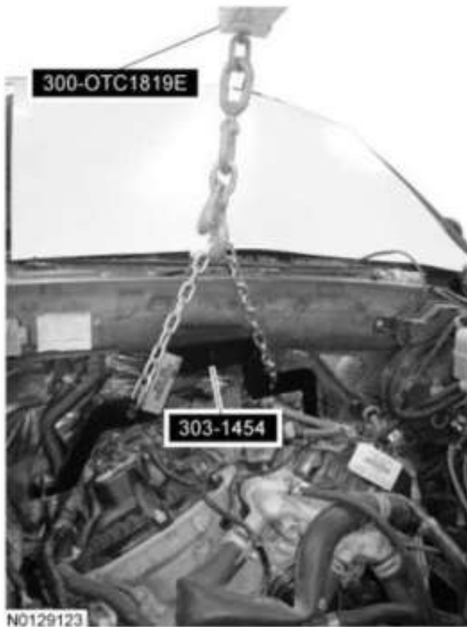
Fig. 490: Lifting Engine Using Floor Crane And Engine Spreader Bar Assembly Courtesy of FORD MOTOR CO.
