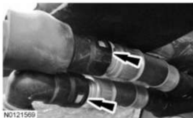
Fig. 460: Locating Heater Hose Couplings Courtesy of FORD MOTOR CO.
