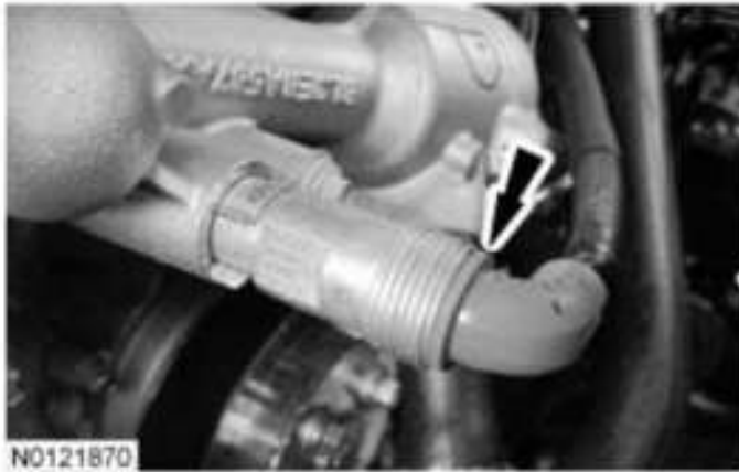
Fig. 453: Locating Block Heater Electrical Connector Courtesy of FORD MOTOR CO.
