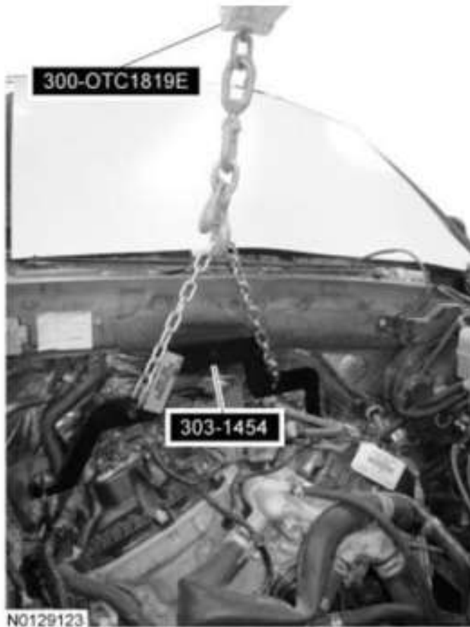
Fig. 487: Lifting Engine Using Floor Crane And Engine Spreader Bar Assembly Courtesy of FORD MOTOR CO.
