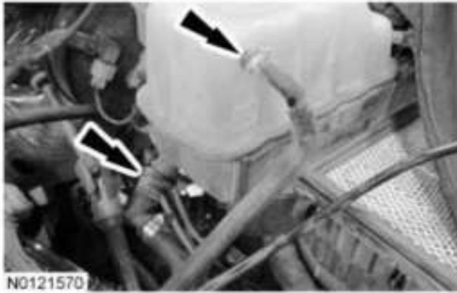
Fig. 461: Locating Coolant Hoses Of Degas Bottle Courtesy of FORD MOTOR CO.
