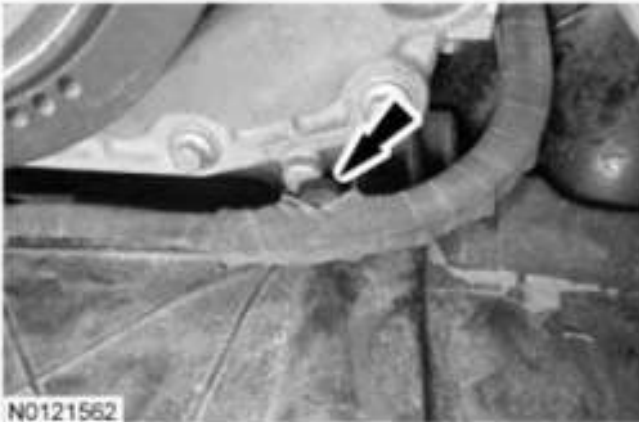
Fig. 457: Identifying Generator Wiring Harness Courtesy of FORD MOTOR CO.
