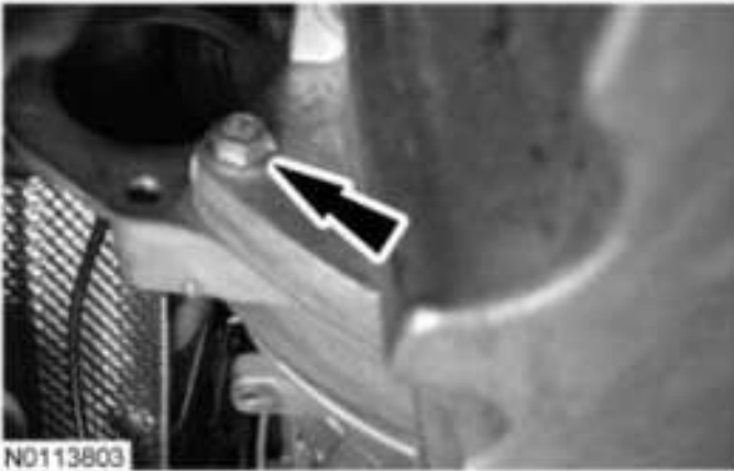
Fig. 478: Locating Oil Pan-To-Bell Housing Bolt Courtesy of FORD MOTOR CO.
