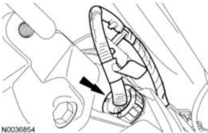
Fig. 469: Locating Transmission Vehicle Harness Connector Courtesy of FORD MOTOR CO.
