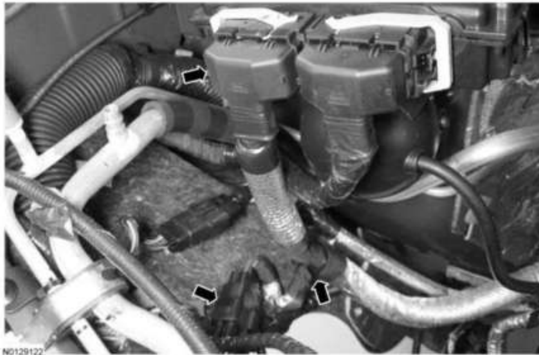
Fig. 459: Locating PCM Electrical Connector And Engine Wire Harness Electrical Connector Courtesy of FORD MOTOR CO.
