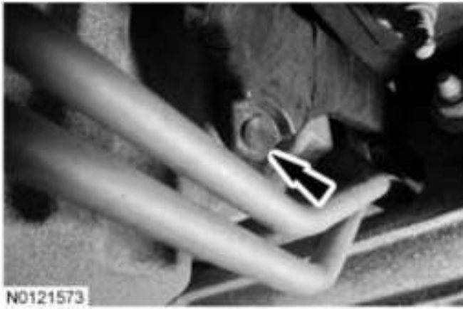
Fig. 470: Locating Starter Motor Wiring Harness Retainer Courtesy of FORD MOTOR CO.
