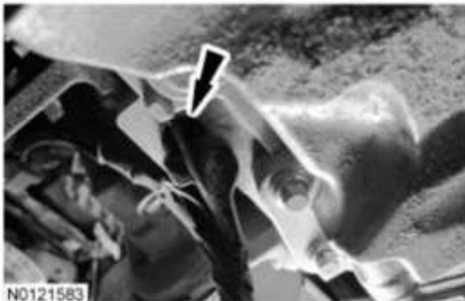
Fig. 489: Locating Generator Wiring Harness Retainer Courtesy of FORD MOTOR CO.
