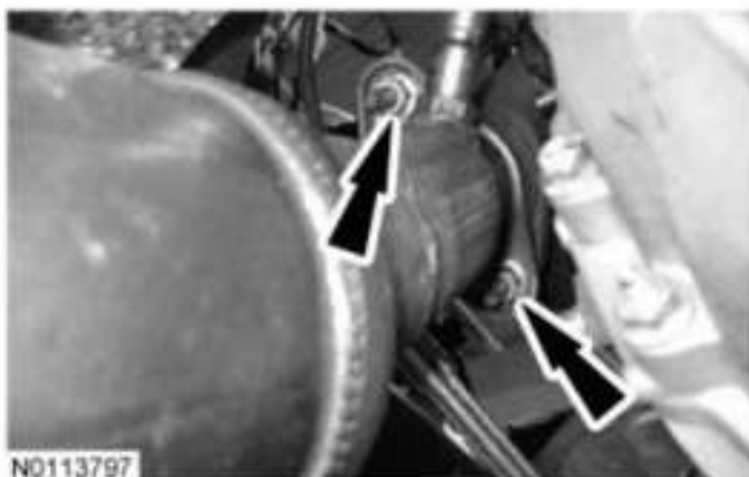
Fig. 474: Locating Catalytic Converter-To-Exhaust Manifold Nuts Courtesy of FORD MOTOR CO.
