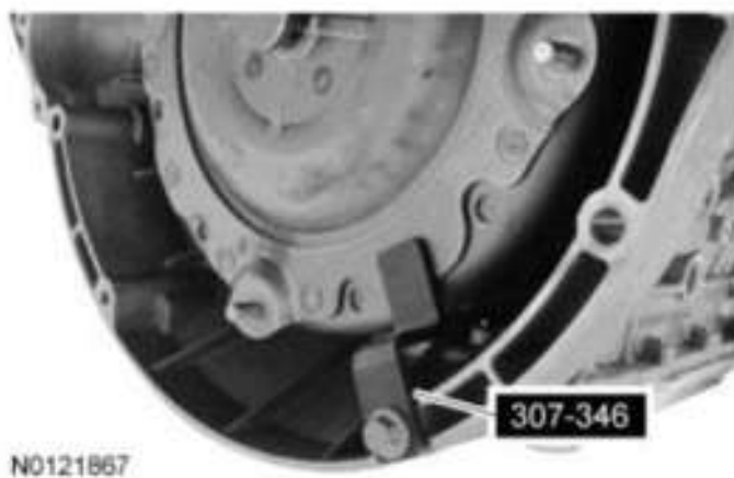
Fig. 491: Locating Torque Converter Retainer Courtesy of FORD MOTOR CO.
