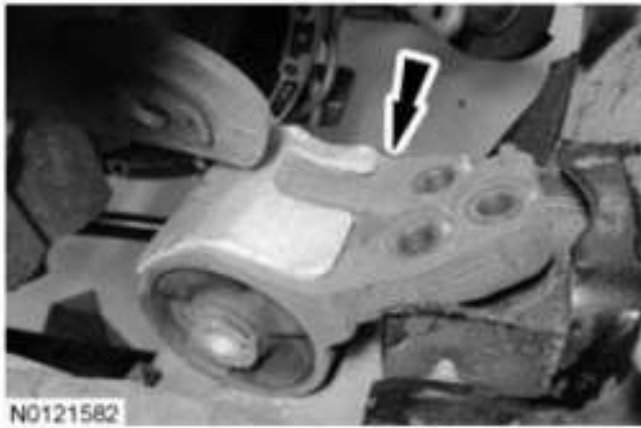
Fig. 488: Locating Engine Support Insulator Courtesy of FORD MOTOR CO.
