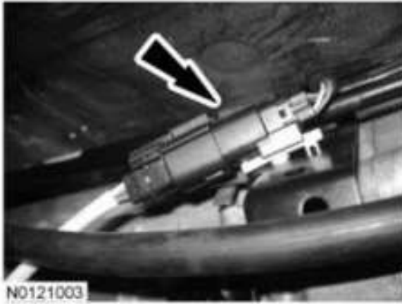
Fig. 468: Locating HO2S Electrical Connector Retainer Courtesy of FORD MOTOR CO.
