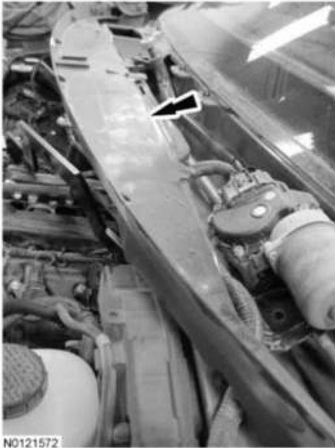
Fig. 464: Locating Cowl Panel Courtesy of FORD MOTOR CO.
