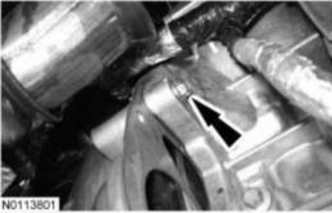
Fig. 477: Locating Engine-To-Bell Housing Bolt Courtesy of FORD MOTOR CO.
