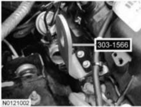
Fig. 484: Locating Right Front Lift Eye Courtesy of FORD MOTOR CO.
