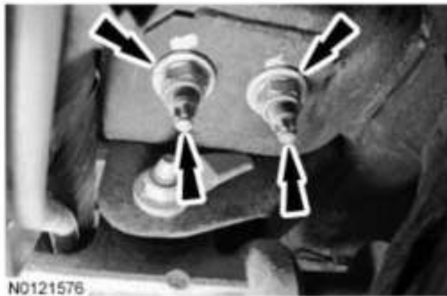
Fig. 476: Locating RH Engine Support Insulator Nuts Courtesy of FORD MOTOR CO.
