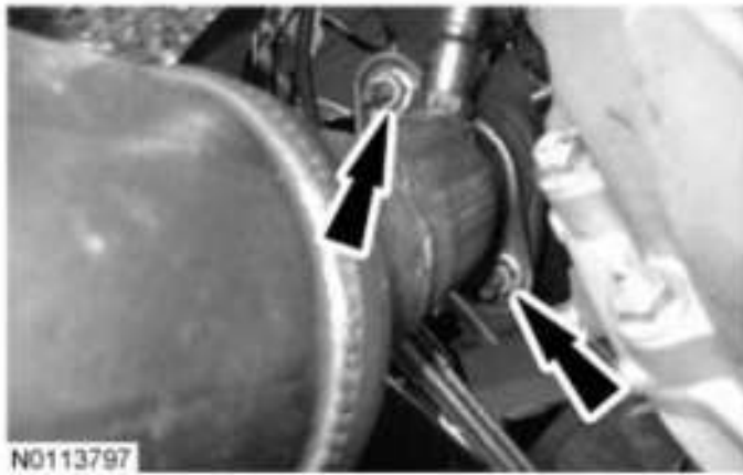
Fig. 876: Locating Catalytic Converter-To-Turbocharger Nuts Courtesy of FORD MOTOR CO.
