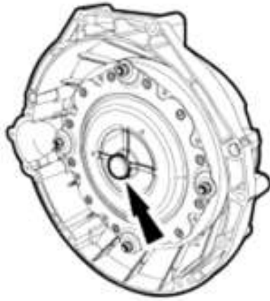
Fig. 856: Locating Torque Converter Pilot Hub Courtesy of FORD MOTOR CO.
