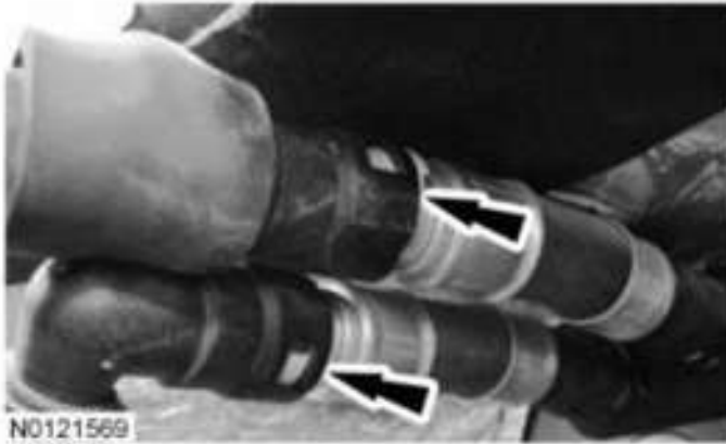
Fig. 890: Locating Heater Hose Couplings Courtesy of FORD MOTOR CO.
