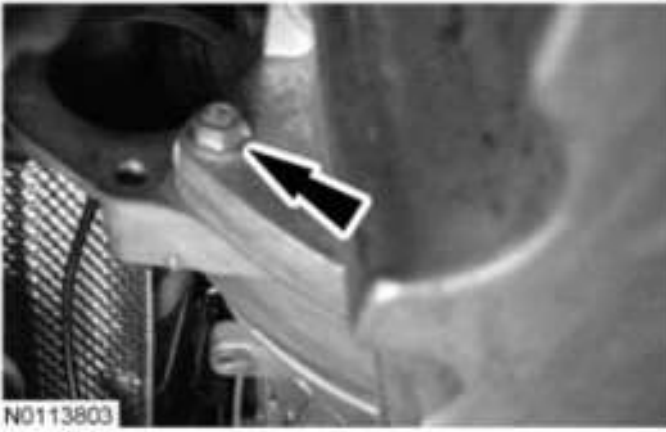
Fig. 871: Locating Oil Pan-To-Bellhousing Bolt Courtesy of FORD MOTOR CO.
