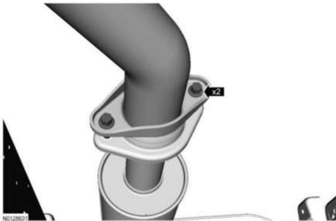
Fig. 877: Locating Exhaust Y-Pipe Dual Catalytic Converter-To-Exhaust Intermediate Pipe Bolts Courtesy of FORD MOTOR CO.
