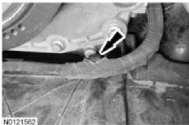
Fig. 893: Identifying Generator Wiring Harness Courtesy of FORD MOTOR CO.
