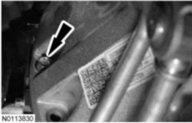
Fig. 869: Locating LH Bellhousing-To-Engine Bolt Courtesy of FORD MOTOR CO.
