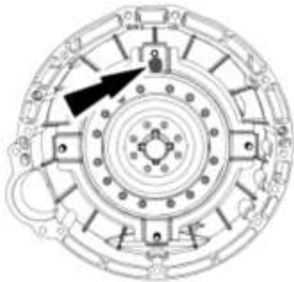
Fig. 857: Locating Torque Converter Stud And Flexplate Hole Courtesy of FORD MOTOR CO.
