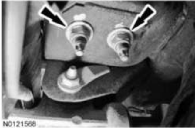
Fig. 867: Locating RH Engine Support Insulator Nuts Courtesy of FORD MOTOR CO.
