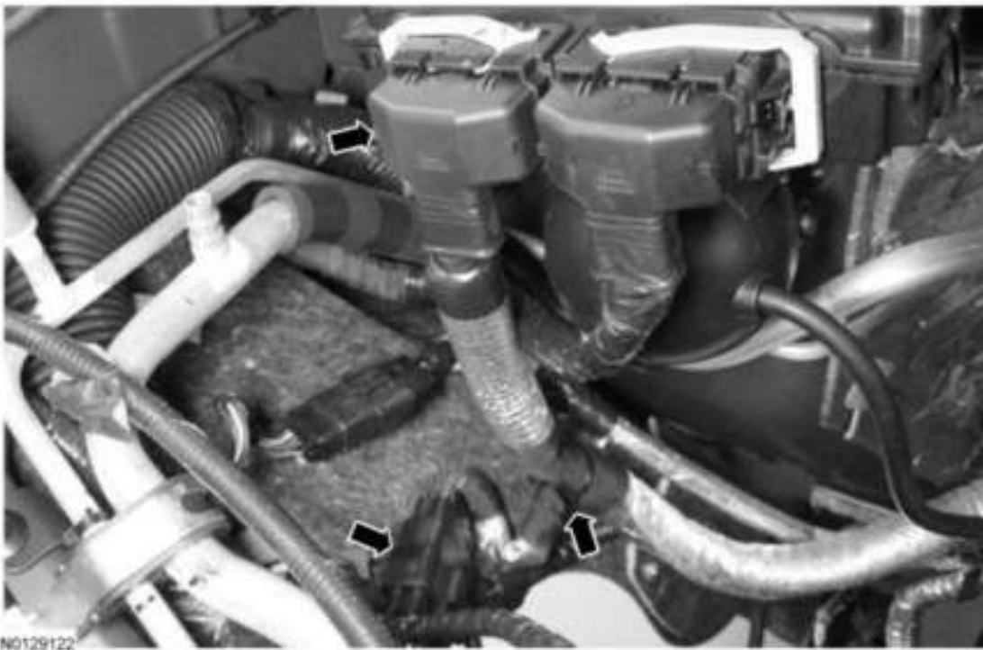
Fig. 891: Locating PCM Electrical Connector And Engine Wire Harness Electrical Connector Courtesy of FORD MOTOR CO.
