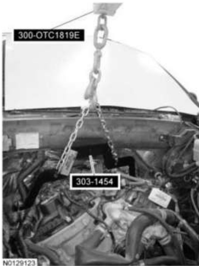
Fig. 860: Lifting Engine Using Floor Crane And Engine Spreader Bar Assembly Courtesy of FORD MOTOR CO.
