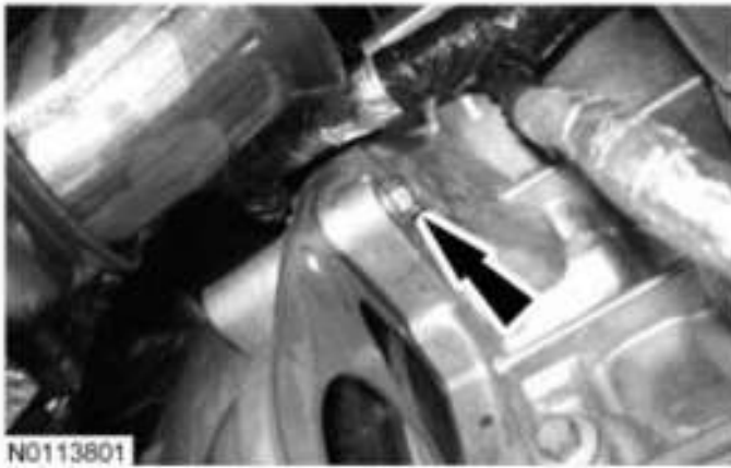
Fig. 870: Locating Engine-To-Bellhousing Bolt Courtesy of FORD MOTOR CO.
