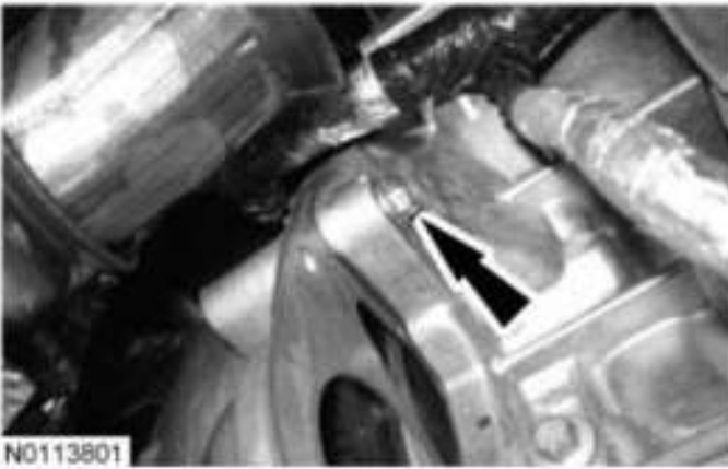
Fig. 872: Locating Engine-To-Bellhousing Bolt Courtesy of FORD MOTOR CO.
