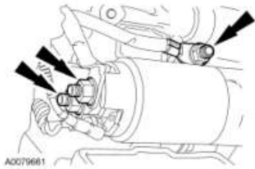
Fig. 125: Locating Positive And Negative Battery Cable Courtesy of FORD MOTOR CO.
