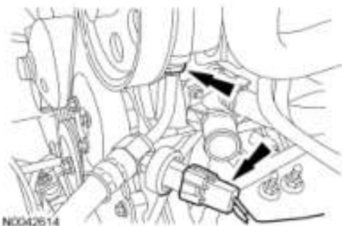
Fig. 122: Locating Power Steering Pressure Switch Electrical Connector And High-Pressure
