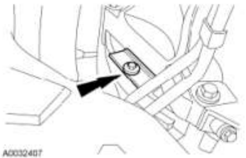
Fig. 133: Locating Transmission Dust Shield Courtesy of FORD MOTOR CO.
