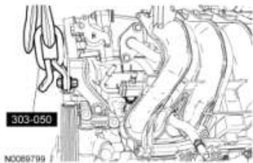
Fig. 152: Installing Engine Lifting Brackets Courtesy of FORD MOTOR CO.
