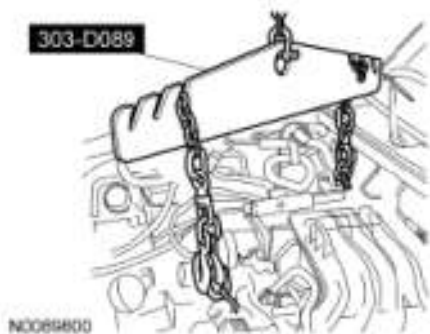
Fig. 153: Supporting Engine With Floor Crane Courtesy of FORD MOTOR CO.
