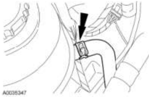
Fig. 117: Locating Engine Coolant Supply Hose Courtesy of FORD MOTOR CO.
