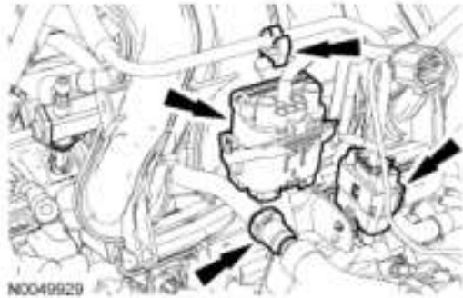
Fig. 123: Locating Evaporative Purge Tube Quick Connect Coupling Courtesy of FORD MOTOR CO.
