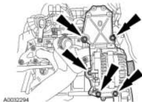
Fig. 161: Locating Accessory Bracket Bolts Courtesy of FORD MOTOR CO.
