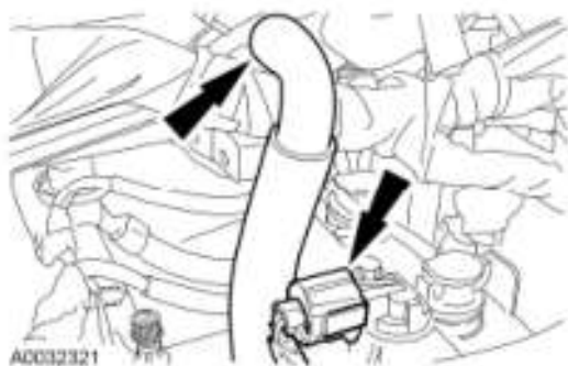
Fig. 173: Locating Camshaft Position Sensor Electrical Connector Courtesy of FORD MOTOR CO.
