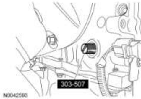
Fig. 284: Identifying Crankshaft Timing Peg Courtesy of FORD MOTOR CO.
