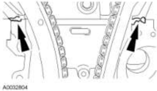
Fig. 275: Identifying Sealant Applying Area Courtesy of FORD MOTOR CO.
