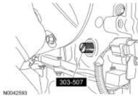
Fig. 292: Identifying Crankshaft Timing Peg Courtesy of FORD MOTOR CO.
