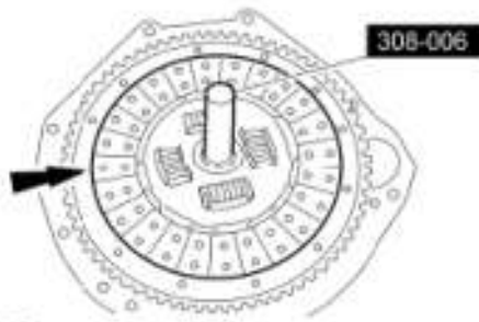
Fig. 331: Identifying Clutch Disc On Flywheel Courtesy of FORD MOTOR CO.
