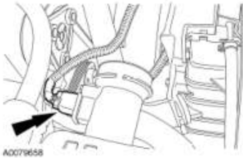
Fig. 365: Locating Mass Air Flow Electrical Connector Courtesy of FORD MOTOR CO.
