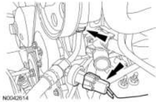
Fig. 362: Locating Power Steering Pressure Switch Electrical Connector And High-Pressure Power Steering Tube Courtesy of FORD MOTOR CO.
