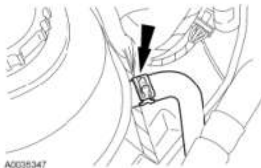
Fig. 367: Locating Engine Coolant Supply Hose Courtesy of FORD MOTOR CO.
