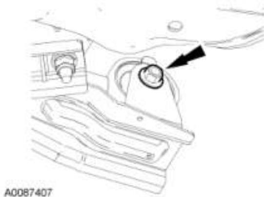
Fig. 219: Locating Rear Roll Restrictor-To-Crossmember Bolt Courtesy of FORD MOTOR CO.
