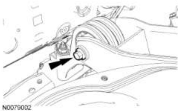
Fig. 223: Locating Rear Transaxle Insulator Through Bolt Courtesy of FORD MOTOR CO.
