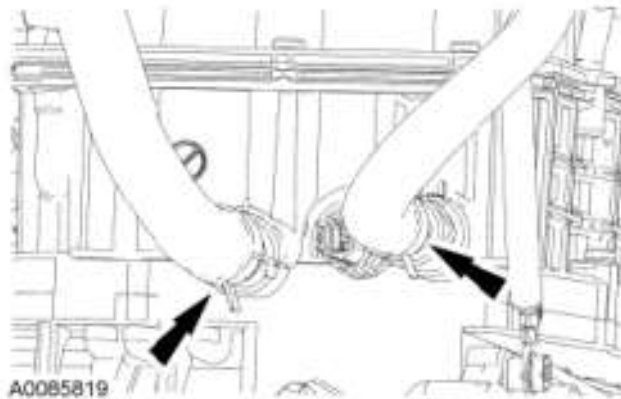
Fig. 206: Locating Transaxle Coolant Hoses Courtesy of FORD MOTOR CO.
