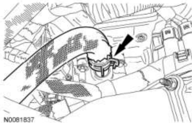
Fig. 200: Locating Coolant Vent Hose Clamp Courtesy of FORD MOTOR CO.
