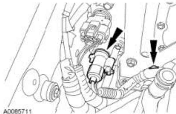
Fig. 201: Locating DC-To-DC Converter Electrical Connector And Wiring Harness Retainers Courtesy of FORD MOTOR CO.
