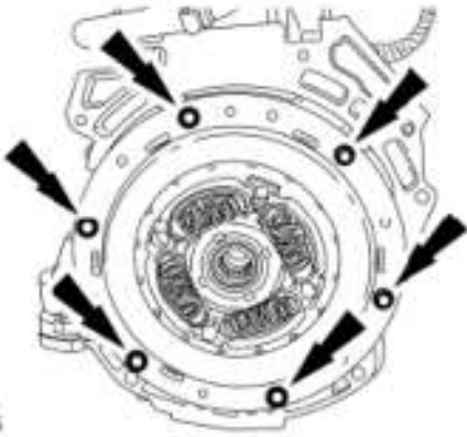
Fig. 235: Locating Transaxle Damper Bolts Courtesy of FORD MOTOR CO.
