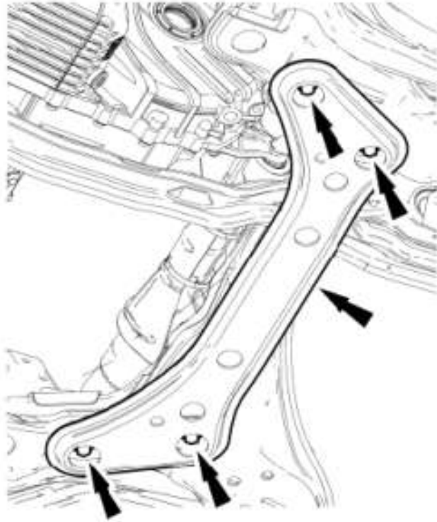
Fig. 176: Locating Lateral Support Crossmember Bolts Courtesy of FORD MOTOR CO.
