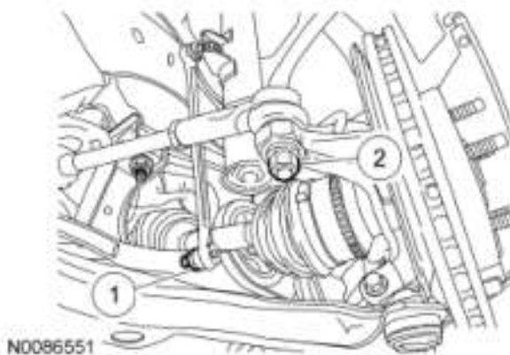
Fig. 180: Identifying Stabilizer Bar Link And Tie-Rod End Retaining Nut Courtesy of FORD MOTOR CO.
