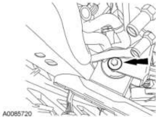
Fig. 218: Locating Lower Insulator Through Bolt Courtesy of FORD MOTOR CO.
