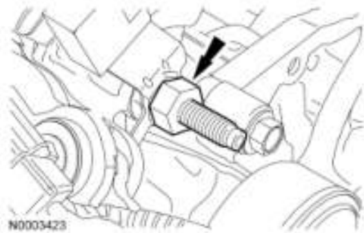
Fig. 310: Identifying RH Radio Ignition Interference Capacitor Stud Bolt Courtesy of FORD MOTOR CO.
