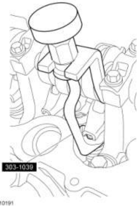
Fig. 337: Compressing Spring Using Special Tool Courtesy of FORD MOTOR CO.
