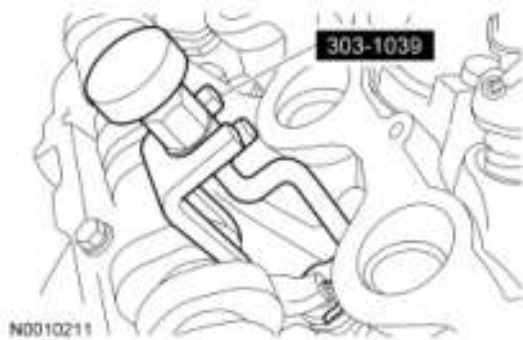
Fig. 335: Identifying Special Tool For Removing/Installing Camshaft Roller Followers Courtesy of FORD MOTOR CO.
