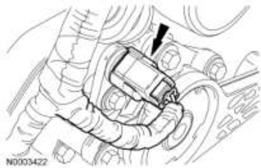
Fig. 309: Identifying RH CMP Sensor Electrical Connector Courtesy of FORD MOTOR CO.
