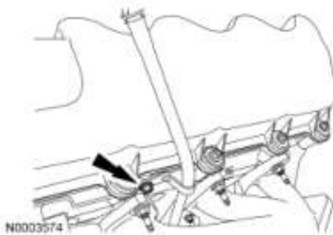
Fig. 319: Locating Oil Level Indicator Tube Bolt Courtesy of FORD MOTOR CO.
