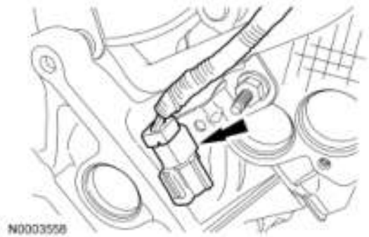
Fig. 313: Locating Electrical Connector Retainer At Coolant Tube Support Bracket Courtesy of FORD MOTOR CO.
