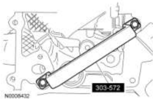
Fig. 352: Identifying Special Tool On Cylinder Head Courtesy of FORD MOTOR CO.
