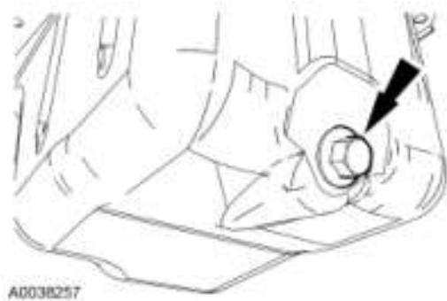
Fig. 292: Locating Drain Plug And Drain Engine Oil Courtesy of FORD MOTOR CO.
