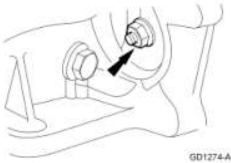
Fig. 288: Locating Torque Converter-To-Flexplate Nuts Courtesy of FORD MOTOR CO.
