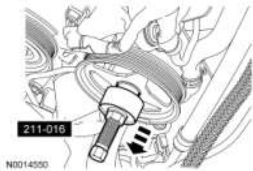
Fig. 282: Removing Power Steering Pump Pulley Using Special Tool Courtesy of FORD MOTOR CO.
