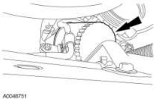
Fig. 295: Removing Oil Filter Courtesy of FORD MOTOR CO.
