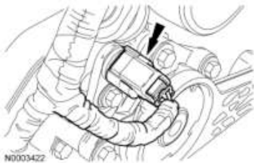
Fig. 366: Identifying RH CMP Sensor Electrical Connector Courtesy of FORD MOTOR CO.
