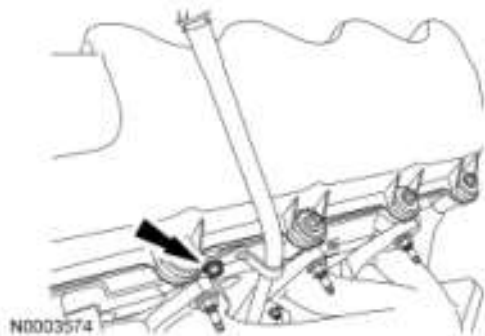
Fig. 378: Locating Oil Level Indicator Tube Bolt Courtesy of FORD MOTOR CO.
