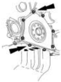
Fig. 361: Identifying Crankshaft Rear Seal Retainer Plate Bolts Courtesy of FORD MOTOR CO.
