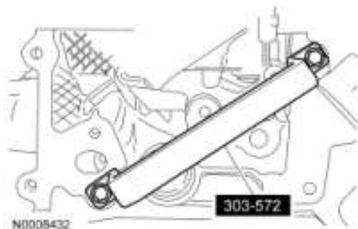
Fig. 413: Identifying Special Tool On Cylinder Head Courtesy of FORD MOTOR CO.
