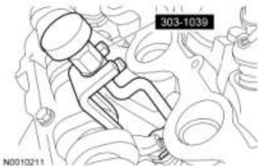
Fig. 402: Identifying Special Tool For Removing/Installing Camshaft Roller Followers Courtesy of FORD MOTOR CO.
