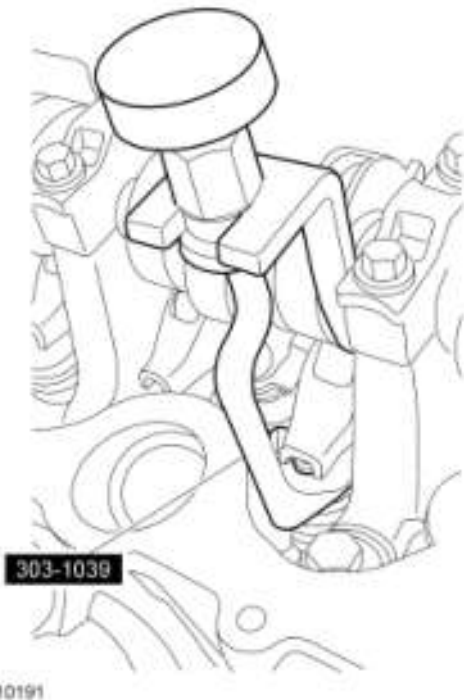
Fig. 404: Compressing Spring Using Special Tool Courtesy of FORD MOTOR CO.
