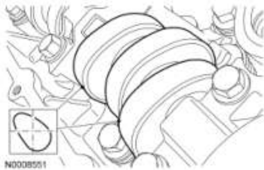
Fig. 400: Identifying Camshaft Lobe Position Courtesy of FORD MOTOR CO.
