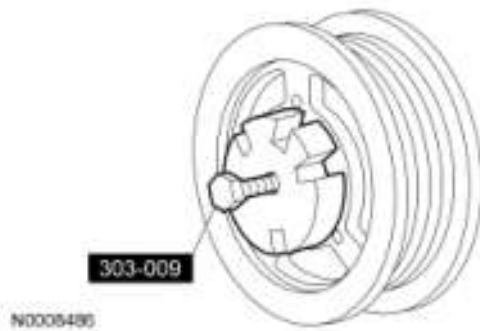
Fig. 393: Removing Crankshaft Pulley Using Special Tool Courtesy of FORD MOTOR CO.
