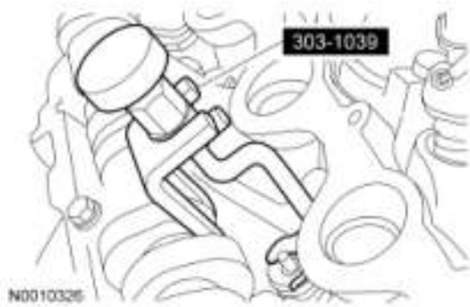
Fig. 431: Compressing Valve Spring With Special Tool Courtesy of FORD MOTOR CO.
