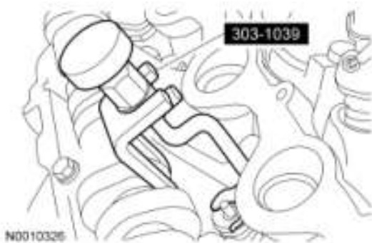
Fig. 428: Compressing Valve Spring With Special Tool Courtesy of FORD MOTOR CO.
