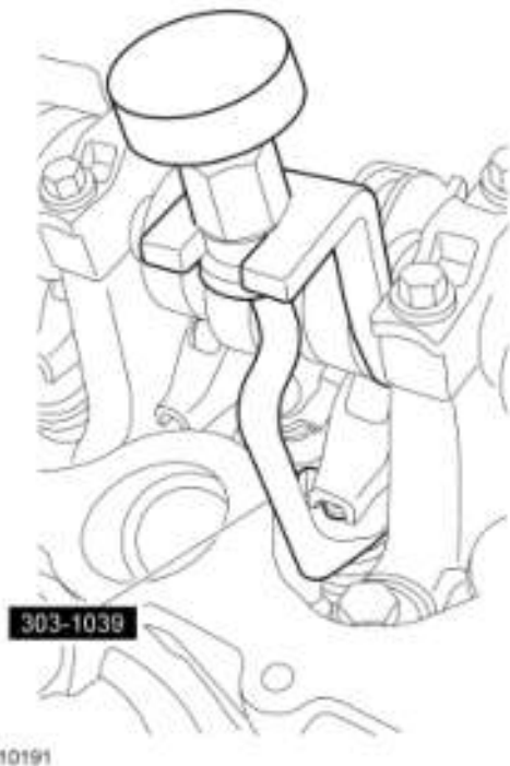
Fig. 480: Compressing Spring Using Special Tool (303-1039) Courtesy of FORD MOTOR CO.
