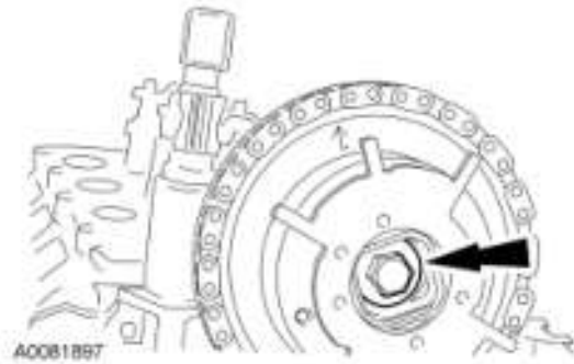
Fig. 463: Identifying Camshaft Phaser And Sprocket Assembly Bolt Courtesy of FORD MOTOR CO.
