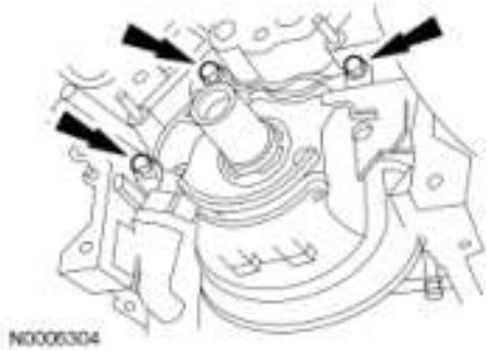
Fig. 453: Locating Oil Pump Bolts Courtesy of FORD MOTOR CO.
