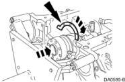
Fig. 444: Installing Front Crankshaft Upper Thrust Washer Courtesy of FORD MOTOR CO.
