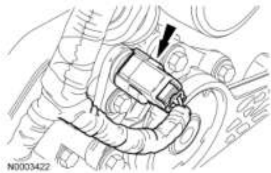
Fig. 522: Identifying RH CMP Sensor Electrical Connector Courtesy of FORD MOTOR CO.
