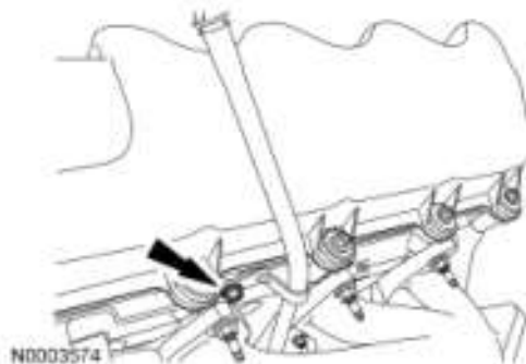
Fig. 509: Installing Oil Level Indicator Tube Courtesy of FORD MOTOR CO.
