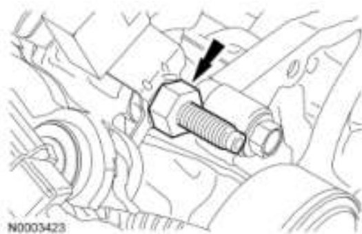
Fig. 521: Identifying RH Radio Ignition Interference Capacitor Stud Bolt Courtesy of FORD MOTOR CO.
