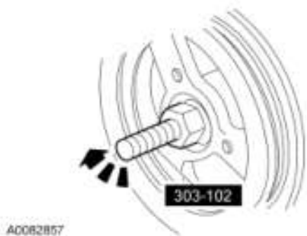
Fig. 491: Using Special Tool To Install Crankshaft Pulley Courtesy of FORD MOTOR CO.
