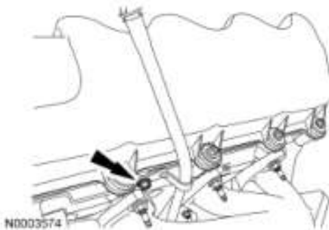
Fig. 608: Installing Oil Level Indicator Tube And Bolt Courtesy of FORD MOTOR CO.
