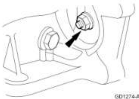
Fig. 539: Locating Torque Converter-To-Flexplate Nuts Courtesy of FORD MOTOR CO.
