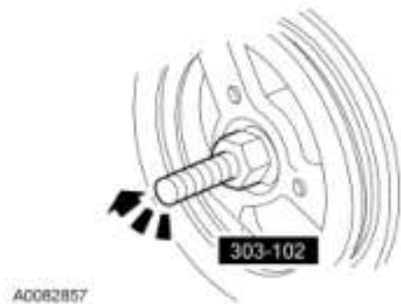
Fig. 613: Using Special Tool To Install Crankshaft Pulley Courtesy of FORD MOTOR CO.
