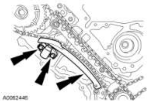
Fig. 593: Identifying RH Timing Chain Tensioner, Tensioner Arm And Bolts Courtesy of FORD MOTOR CO.
