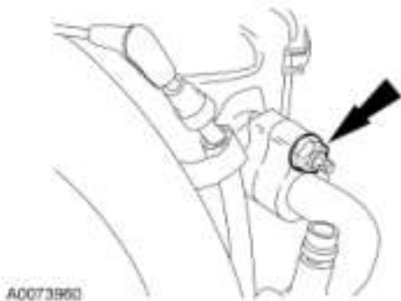
Fig. 560: Using New O-Ring Seal To Connect A/C Manifold And Tube Assembly And Install Nut Courtesy of FORD MOTOR CO.
