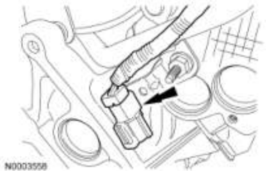
Fig. 625: Locating Electrical Connector Retainer At Coolant Tube Support Bracket Courtesy of FORD MOTOR CO.
