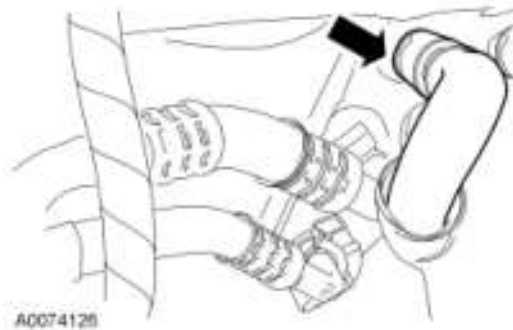
Fig. 562: Connecting Heater Hose Courtesy of FORD MOTOR CO.
