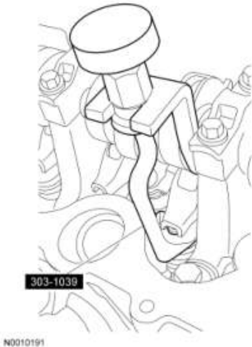
Fig. 597: Compressing Spring Using Special Tool Courtesy of FORD MOTOR CO.
