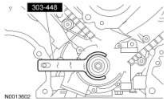
Fig. 567: Positioning Crankshaft With Special Tool Courtesy of FORD MOTOR CO.
