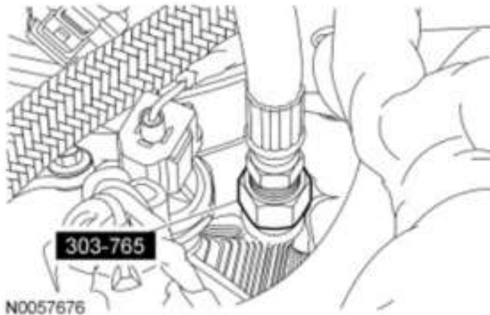
Fig. 6: Identifying High-Pressure Pump Test Adapter Courtesy of FORD MOTOR CO.
