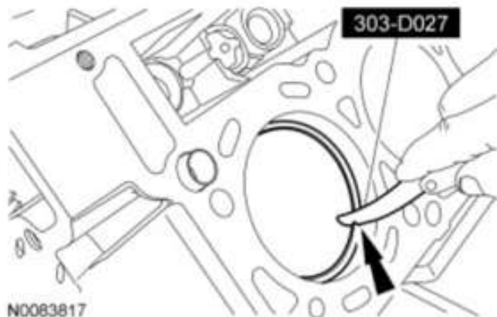
Fig. 36: Measuring Gap Between Ends Of Each Piston Ring Courtesy of FORD MOTOR CO.
