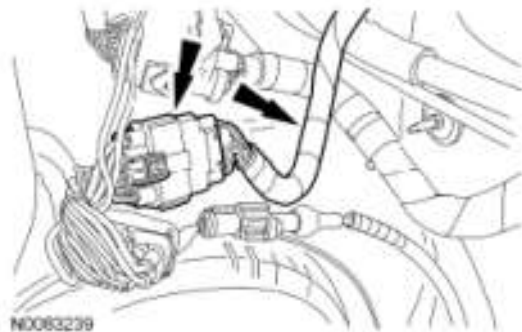
Fig. 236: Locating Engine Harness Electrical Connector Courtesy of FORD MOTOR CO.
