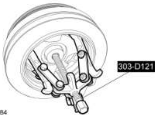
Fig. 261: Identifying Jaw Puller On Crankshaft Pulley Courtesy of FORD MOTOR CO.
