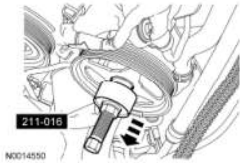
Fig. 234: Removing Power Steering Pump Pulley Using Power Steering Pump Pulley Remover Courtesy of FORD MOTOR CO.
