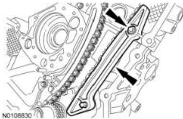
Fig. 276: Locating LH Timing Chain Guide And Mounting Bolt Courtesy of FORD MOTOR CO.
