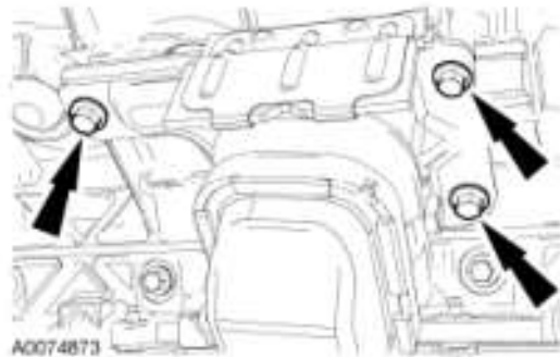
Fig. 308: Locating RH Engine Support Insulator Bolts Courtesy of FORD MOTOR CO.
