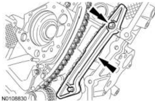
Fig. 485: Locating Bolt And LH Timing Chain Guide Courtesy of FORD MOTOR CO.
