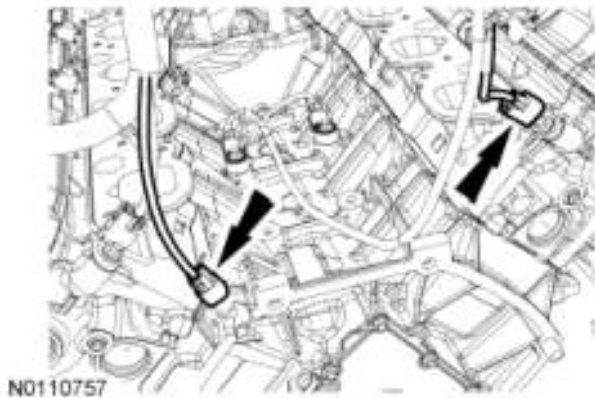
Fig. 517: Locating LH And RH Camshaft Position Electrical Connectors Courtesy of FORD MOTOR CO.
