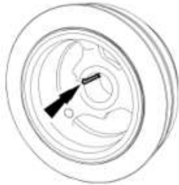
Fig. 502: Locating Woodruff Key Slot In Crankshaft Pulley Courtesy of FORD MOTOR CO.
