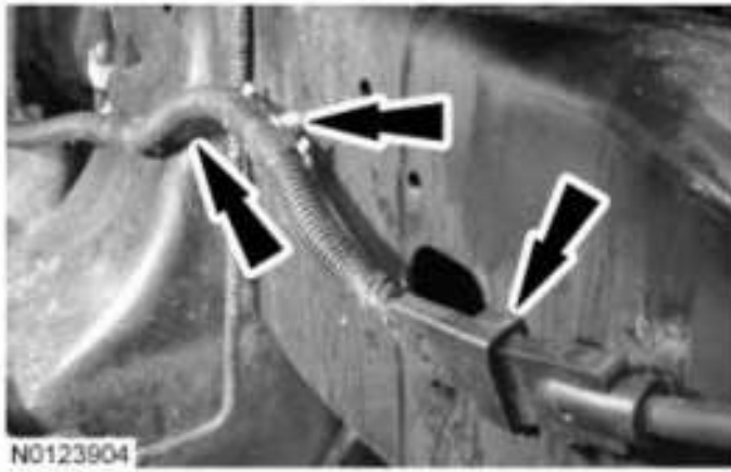
Fig. 481: Locating Wiring Harness Retainers Courtesy of FORD MOTOR CO.
