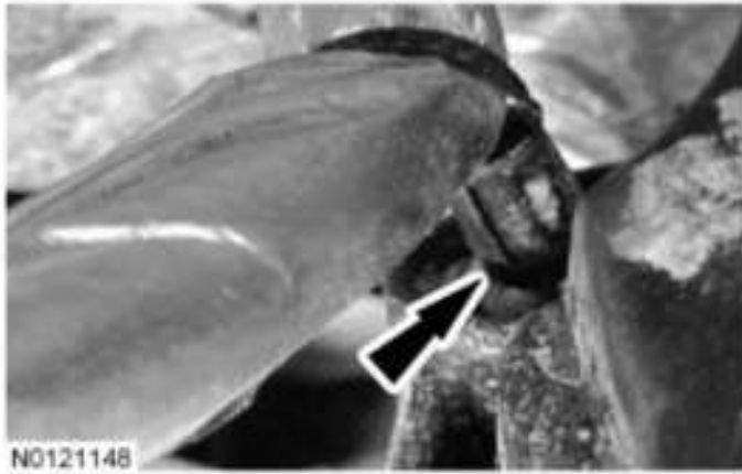
Fig. 476: Locating PCM Wiring Harness Retainer Courtesy of FORD MOTOR CO.
