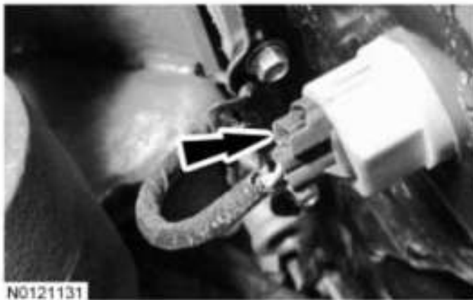
Fig. 497: Locating Oil Level Sensor Electrical Connector Courtesy of FORD MOTOR CO.
