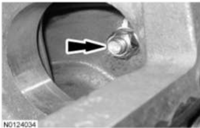
Fig. 484: Locating Torque Converter-To-Flexplate Nuts Courtesy of FORD MOTOR CO.
