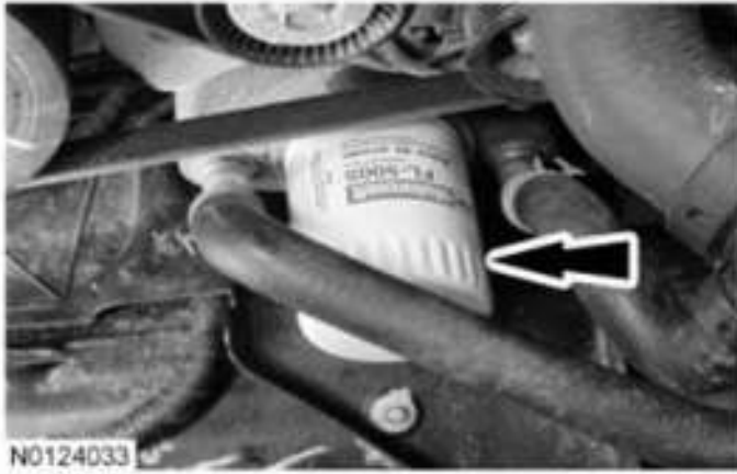
Fig. 489: Locating Engine Oil Filter Courtesy of FORD MOTOR CO.
