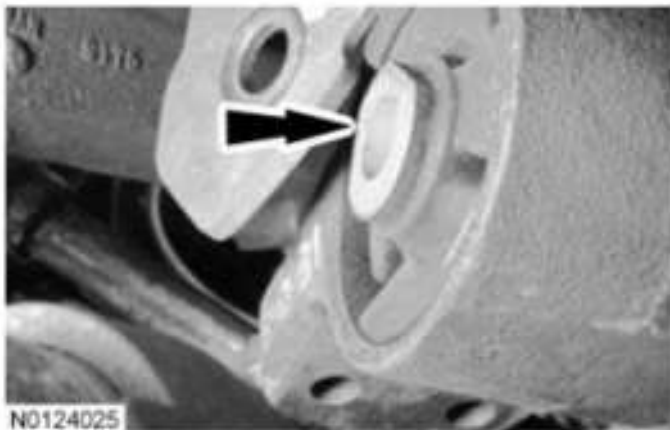
Fig. 502: Locating Engine Support Insulator Courtesy of FORD MOTOR CO.
