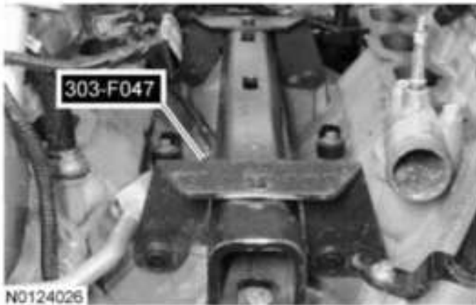
Fig. 500: Locating Engine Lifting Bracket Courtesy of FORD MOTOR CO.
