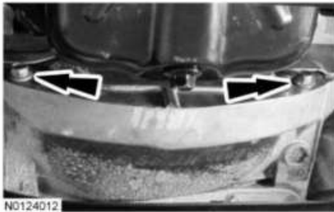
Fig. 482: Locating Flexplate Inspection Cover Mounting Bolts Courtesy of FORD MOTOR CO.
