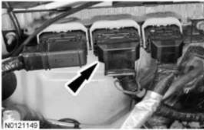
Fig. 474: Locating PCM Electrical Connector Courtesy of FORD MOTOR CO.
