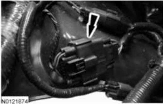
Fig. 475: Locating Engine Harness Electrical Connector Courtesy of FORD MOTOR CO.
