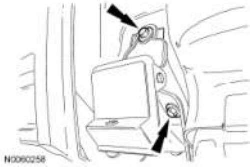
Fig. 241: Locating Transmission Support Crossmember Nuts And Bolts Courtesy of FORD MOTOR CO.
