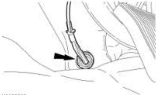
Fig. 227: Locating LH Exhaust Heat Shield Bolt Courtesy of FORD MOTOR CO.
