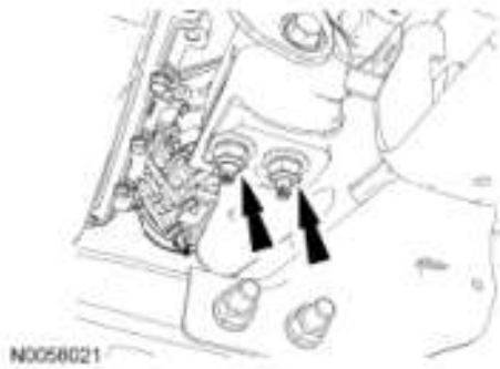
Fig. 168: Locating Transmission Fluid Filter Courtesy of FORD MOTOR CO.
