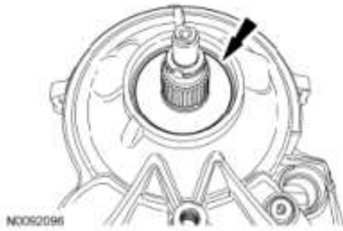
Fig. 178: Locating Slip Plane Washer Courtesy of FORD MOTOR CO.
