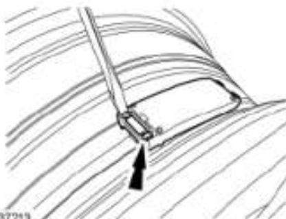
Fig. 138: Locating Transmission Fluid Filter Seal Courtesy of FORD MOTOR CO.
