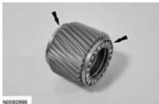
Fig. 329: Locating Top And Bottom Roller Bearings
