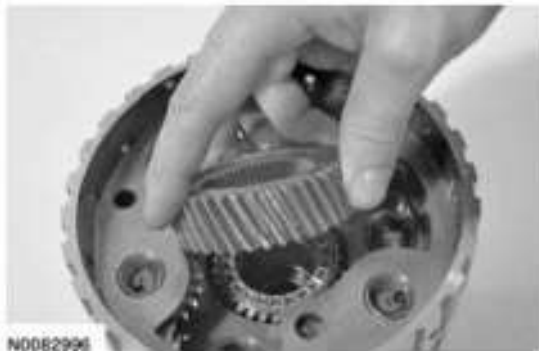
Fig. 327: Removing Low/Reverse Sun Gear Courtesy of FORD MOTOR CO.
