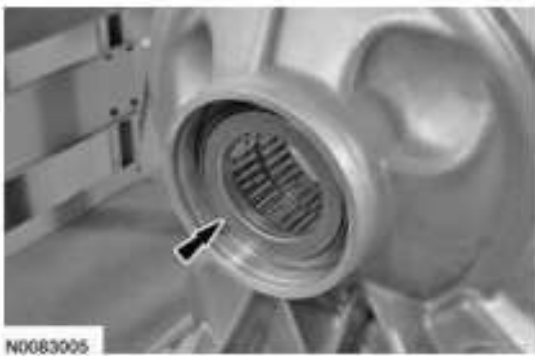
Fig. 337: Locating Thrust Bearing Courtesy of FORD MOTOR CO.
