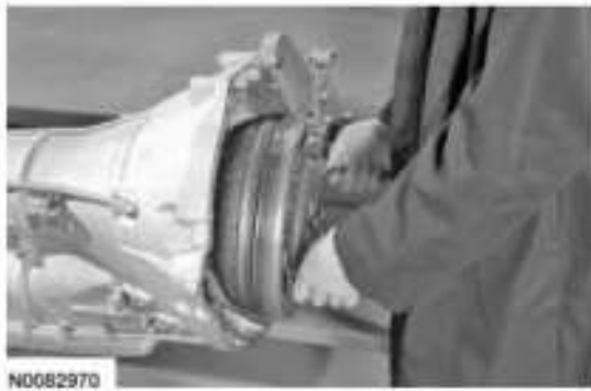
Fig. 301: Removing Torque Converter Courtesy of FORD MOTOR CO.
