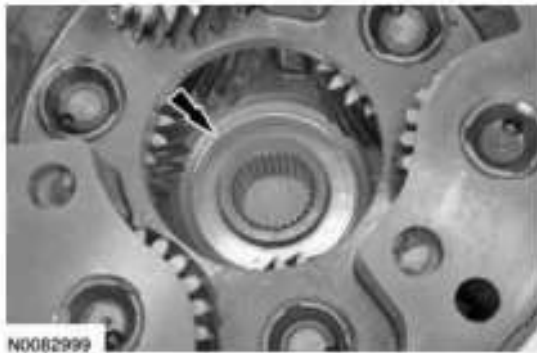
Fig. 330: Locating Roller Bearing Race In Bottom Of Carrier Courtesy of FORD MOTOR CO.
