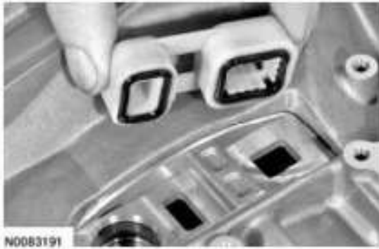
Fig. 309: Removing Rubber Adapter And Fluid Filter Seal Courtesy of FORD MOTOR CO.
