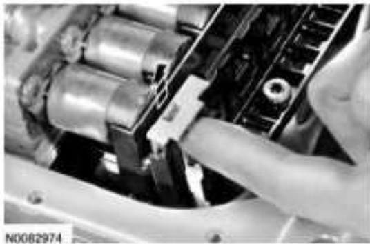
Fig. 305: Pressing Release Tab And Lift Up On Bulkhead Connector Retainer Courtesy of FORD MOTOR CO.
