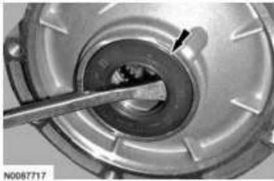
Fig. 342: Removing Output Shaft Seal Courtesy of FORD MOTOR CO.
