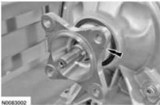
Fig. 333: Locating Extension Housing Flange Seal And Output Shaft Flange Courtesy of FORD MOTOR CO.
