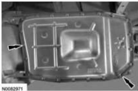
Fig. 302: Locating Transmission Fluid Pan And Bolts Courtesy of FORD MOTOR CO.
