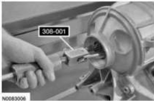
Fig. 338: Removing Thrust Bearing Spacer Courtesy of FORD MOTOR CO.
