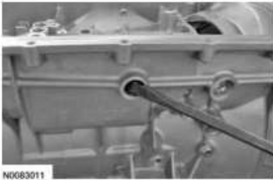
Fig. 347: Removing Manual Control Lever Seal Courtesy of FORD MOTOR CO.
