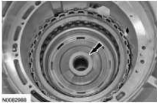
Fig. 320: Locating Caged Roller Bearing Courtesy of FORD MOTOR CO.
