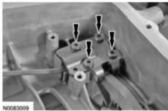
Fig. 345: Locating Park Rod Actuating Plate Courtesy of FORD MOTOR CO.
