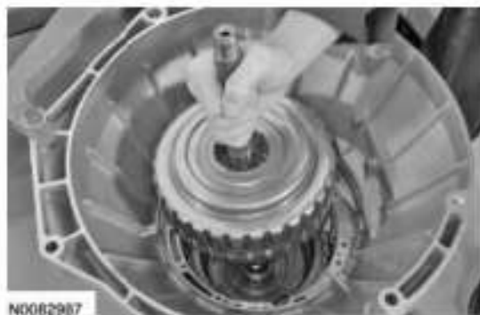
Fig. 319: Removing Forward (Clutch A)/Overdrive (Clutch E) Clutch Assembly Courtesy of FORD MOTOR CO.
