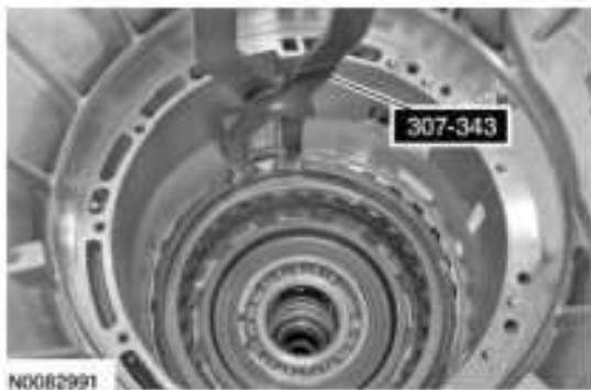
Fig. 322: Removing Center Support Snap Ring Courtesy of FORD MOTOR CO.
