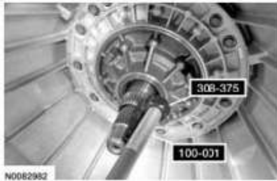
Fig. 313: Removing Pump Seal Courtesy of FORD MOTOR CO.
