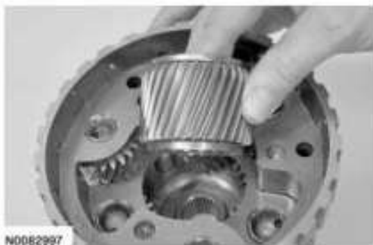
Fig. 328: Removing Sun Gear Into Planet Assembly Courtesy of FORD MOTOR CO.
