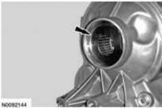
Fig. 336: Locating Slip Plane Washer Courtesy of FORD MOTOR CO.
