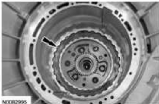
Fig. 326: Locating Planet Carrier And Low/Reverse Clutch Pack Courtesy of FORD MOTOR CO.
