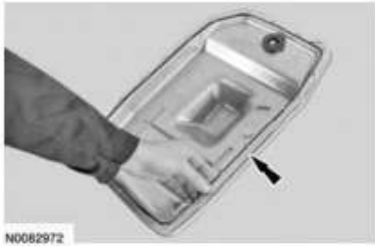
Fig. 303: Locating Transmission Fluid Pan Gasket Courtesy of FORD MOTOR CO.
