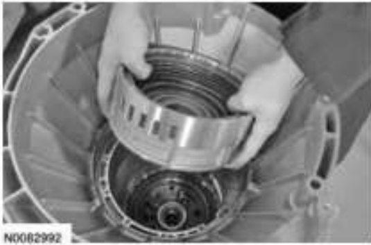
Fig. 323: Removing Center Support And T6 Bearing Courtesy of FORD MOTOR CO.
