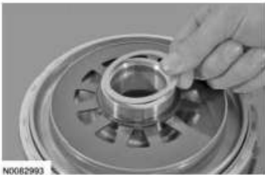
Fig. 324: Removing Selective Shim From Center Support Courtesy of FORD MOTOR CO.
