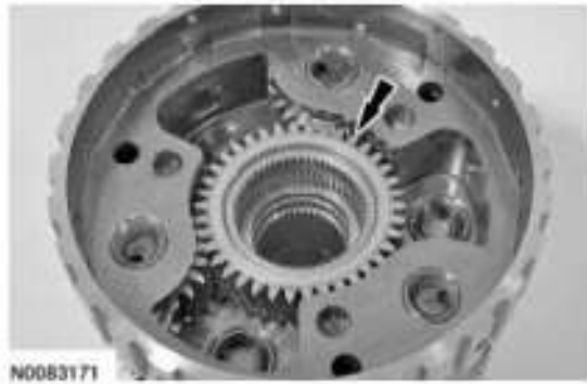
Fig. 569: Locating Low/Reverse Sun Gear And Race In Planet Carrier Courtesy of FORD MOTOR CO.
