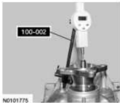
Fig. 576: Identifying Dial Indicator Gauge With Holding Fixture 100-002 On Transmission Case Courtesy of FORD MOTOR CO.
