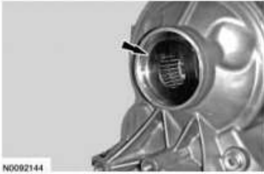
Fig. 557: Locating Slip Plane Washer Courtesy of FORD MOTOR CO.
