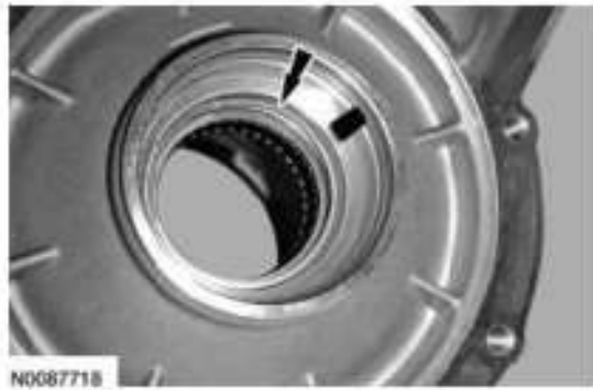
Fig. 550: Locating Snap Ring Courtesy of FORD MOTOR CO.
