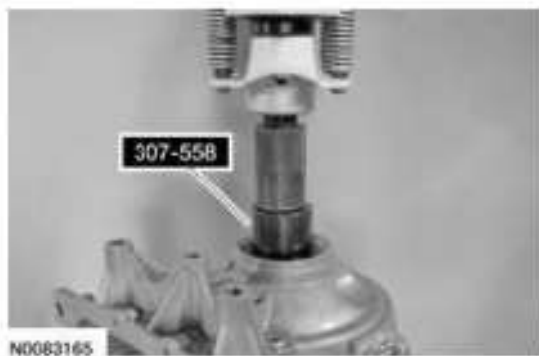
Fig. 555: Pressing Thrust Bearing Spacer Using Needle Bearing Installer 307-558 Courtesy of FORD MOTOR CO.
