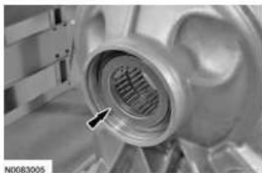
Fig. 556: Locating T12 Thrust Bearing Courtesy of FORD MOTOR CO.
