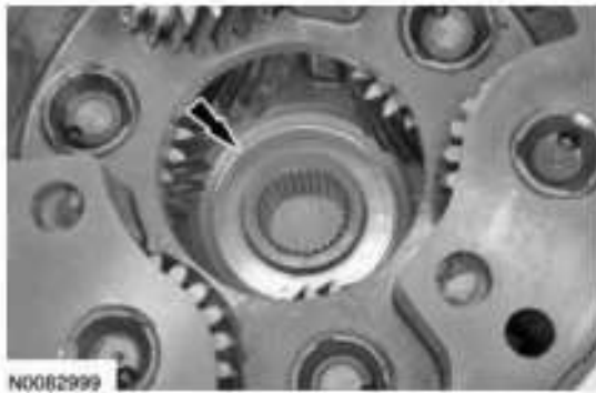
Fig. 566: Locating T9 Roller Bearing Race In Bottom Of Carrier Courtesy of FORD MOTOR CO.
