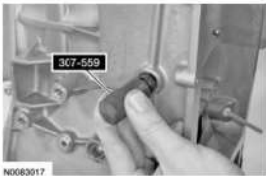
Fig. 542: Installing Manual Control Lever Shaft Seal Courtesy of FORD MOTOR CO.
