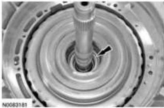
Fig. 585: Locating Selective Pump Washer Courtesy of FORD MOTOR CO.
