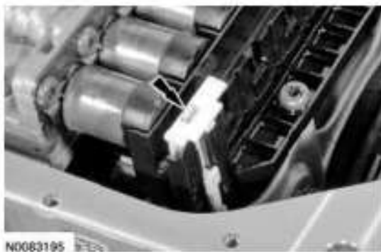
Fig. 603: Locating Outer Shell Of Bulkhead Electrical Connector Courtesy of FORD MOTOR CO.
