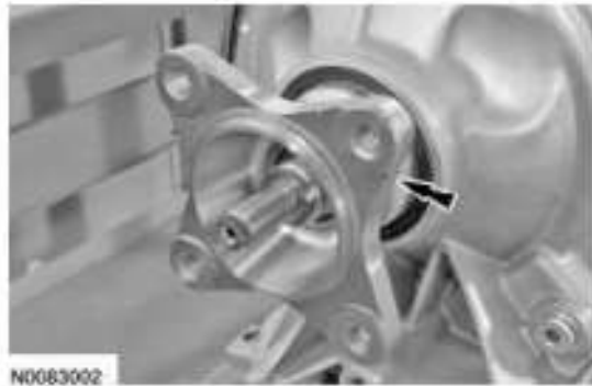
Fig. 563: Locating Extension Housing Flange Seal And Output Shaft Flange Courtesy of FORD MOTOR CO.
