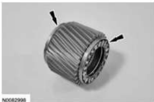
Fig. 567: Locating Top T8 And Bottom T9 Roller Bearings Courtesy of FORD MOTOR CO.
