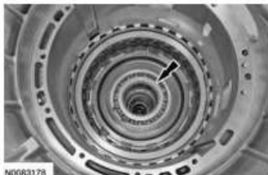
Fig. 581: Locating T6 Thrust Bearing Courtesy of FORD MOTOR CO.
