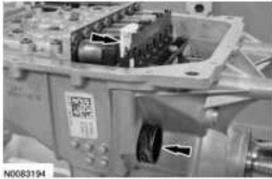
Fig. 602: Locating Tab And Bulkhead Electrical Connector Courtesy of FORD MOTOR CO.
