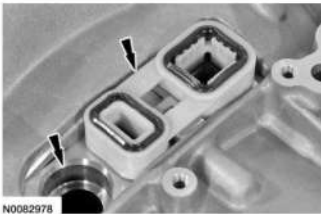
Fig. 597: Locating Rubber Adapter Courtesy of FORD MOTOR CO.
