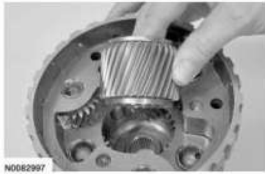
Fig. 568: Installing Sun Gear Into Planet Assembly Courtesy of FORD MOTOR CO.
