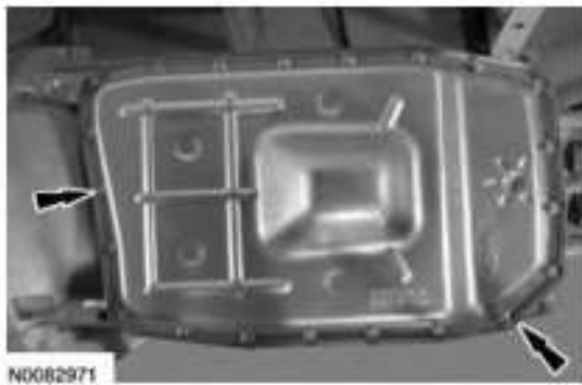
Fig. 606: Locating Transmission Fluid Pan And Bolts Courtesy of FORD MOTOR CO.
