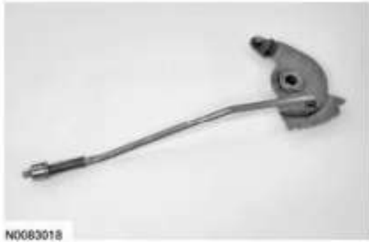
Fig. 543: Identifying Manual Valve Detent Lever Assembly And Park Pawl Actuator Rod Courtesy of FORD MOTOR CO.
