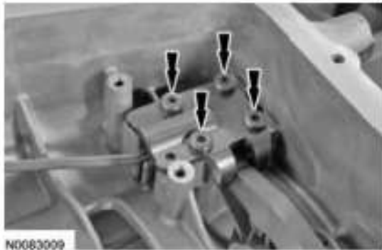
Fig. 547: Locating Park Rod Actuating Plate Courtesy of FORD MOTOR CO.
