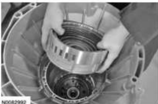
Fig. 574: Installing Center Support Into Case Courtesy of FORD MOTOR CO.
