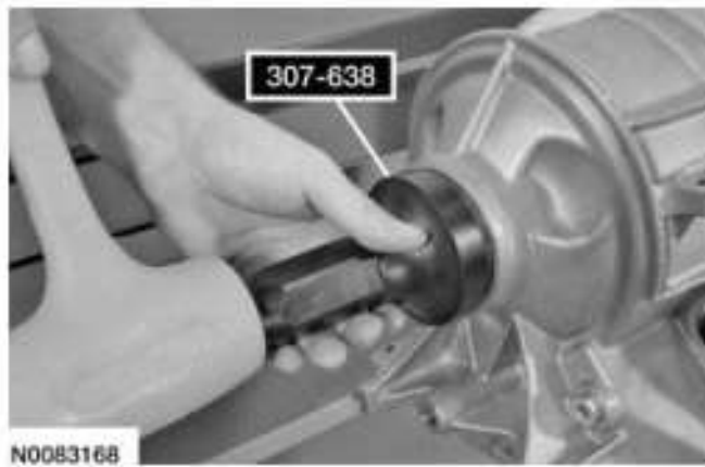
Fig. 562: Tapping Output Shaft Seal Courtesy of FORD MOTOR CO.
