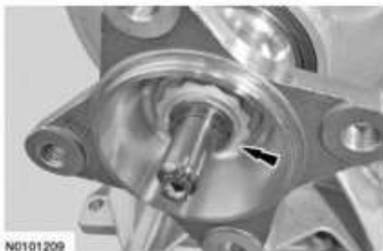
Fig. 564: Locating Output Shaft Flange Nut Courtesy of FORD MOTOR CO.
