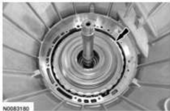
Fig. 584: Locating Forward And Overdrive Clutch Assembly Courtesy of FORD MOTOR CO.
