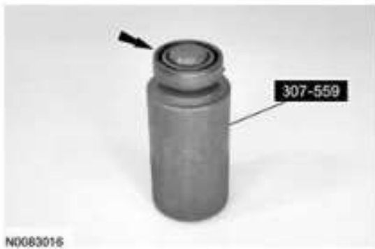
Fig. 541: Locating Manual Control Lever Shaft Seal On Shifter Fluid Seal Installer 307-559 Courtesy of FORD MOTOR CO.
