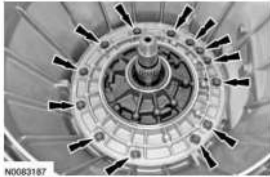
Fig. 592: Locating Front Pump Bolts Courtesy of FORD MOTOR CO.
