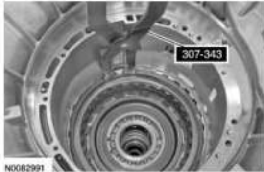
Fig. 575: Installing Center Support Snap Ring Courtesy of FORD MOTOR CO.
