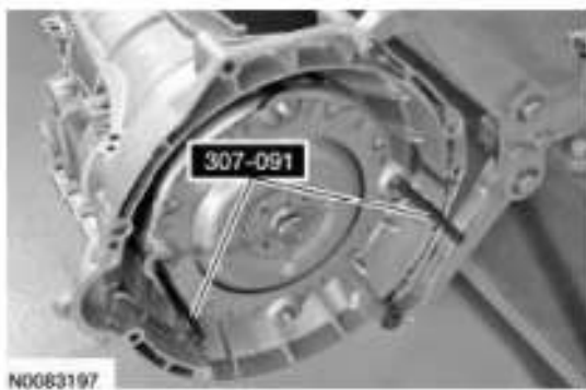
Fig. 607: Identifying Torque Converter Handle 307-091 On Torque Converter Courtesy of FORD MOTOR CO.
