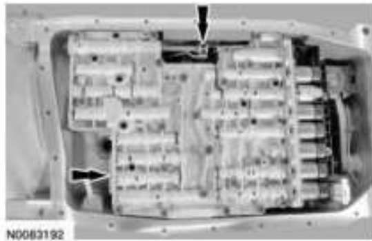
Fig. 600: Locating Manual Valve And Rubber Feed Tubes Courtesy of FORD MOTOR CO.
