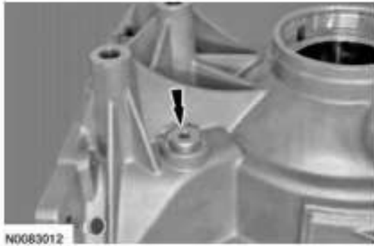
Fig. 540: Locating Park Pawl Pin Bolt Courtesy of FORD MOTOR CO.
