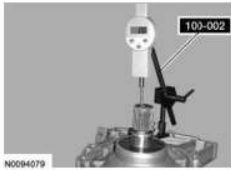
Fig. 579: Identifying Dial Indicator Gauge With Holding Fixture 100-002 On Transmission Case Courtesy of FORD MOTOR CO.
