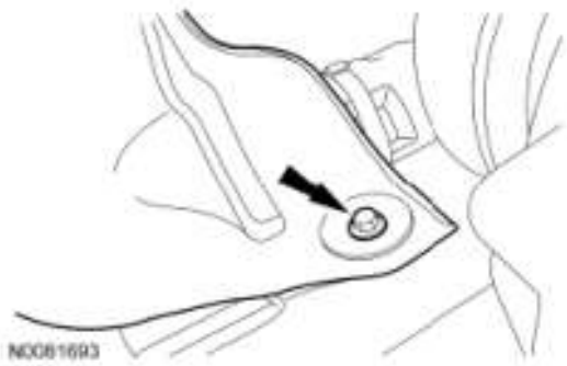
Fig. 623: Identifying Rubber Torque Converter Access Plug Courtesy of FORD MOTOR CO.
