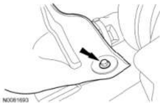
Fig. 617: Locating Plastic Starter Motor Electrical Connector Cap Courtesy of FORD MOTOR CO.
