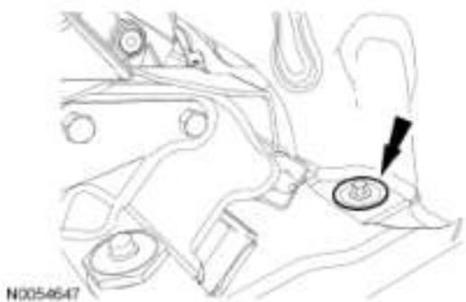
Fig. 624: Identifying Flexplate Inspection Cover Bolts Courtesy of FORD MOTOR CO.
