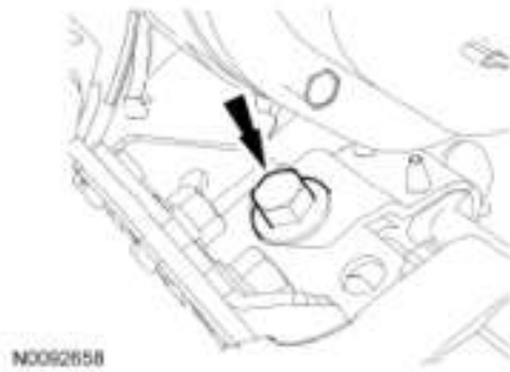
Fig. 616: Identifying Starter Motor Electrical Connectors Bolts Courtesy of FORD MOTOR CO.
