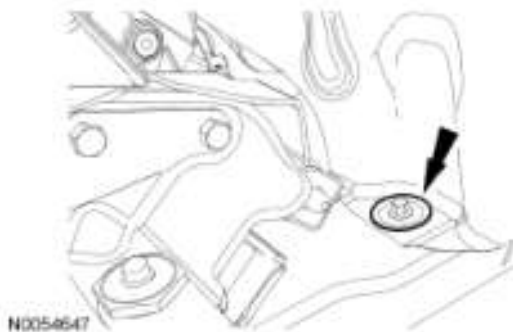
Fig. 618: Identifying Transmission Fluid Cooler Tube Bracket Courtesy of FORD MOTOR CO.
