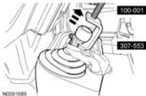
Fig. 4: Removing Shift Lever Knob Courtesy of FORD MOTOR CO.
