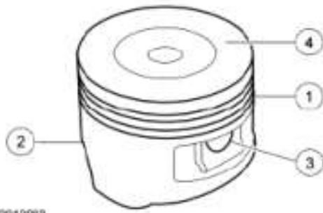
Fig. 19: Identifying Ring Lands, Skirts And Pin Bosses Courtesy of FORD MOTOR CO.
