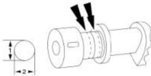
Fig. 5: Measuring Camshaft Journal Courtesy of FORD MOTOR CO.
