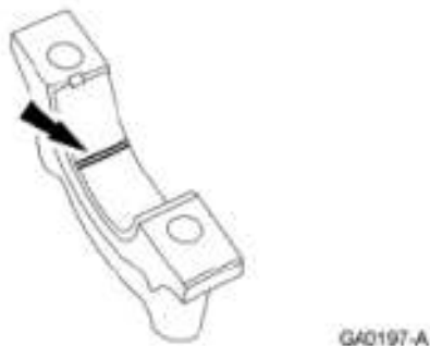
Fig. 13: Laying Piece Of Plastigage Across Face Of Crankshaft Main Bearing Surface Courtesy of FORD MOTOR CO.
