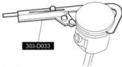
Fig. 20: Cleaning Piston Ring Grooves Courtesy of FORD MOTOR CO.
