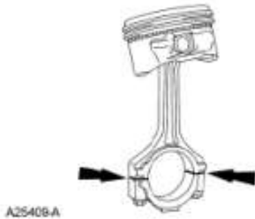
Fig. 28: Identifying Connecting Rod Large End Installation Position Courtesy of FORD MOTOR CO.
