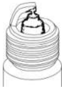
Fig. 61: Identifying Spark Plug For Bridged Gap Courtesy of FORD MOTOR CO.
