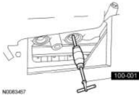
Fig. 58: Removing Core Plug
