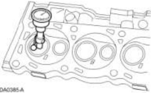
Fig. 53: Checking Valve Seat Runout Courtesy of FORD MOTOR CO.
