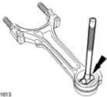
Fig. 30: Checking Connecting Rod Bushing Diameter Courtesy of FORD MOTOR CO.
