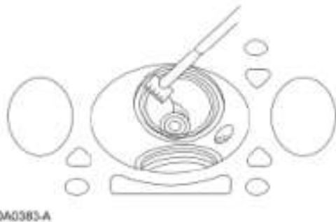
Fig. 52: Measuring Valve Seat Width Courtesy of FORD MOTOR CO.
