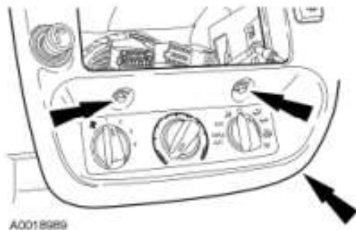
Fig. 24: Locating Instrument Panel Finish Panel Screws Courtesy of FORD MOTOR CO.
