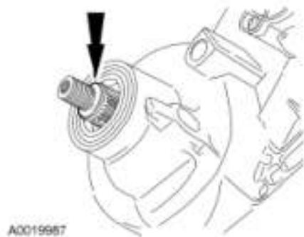
Fig. 8: Locating Oil Seal On Rear Output Shaft Courtesy of FORD MOTOR CO.
