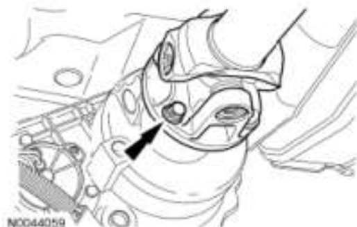
Fig. 13: Locating Driveshaft-To-Flange Bolts Courtesy of FORD MOTOR CO.
