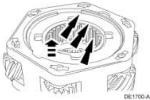
Fig. 48: Locating Snap Ring, Thrust Plate And Sun Gear Courtesy of FORD MOTOR CO.
