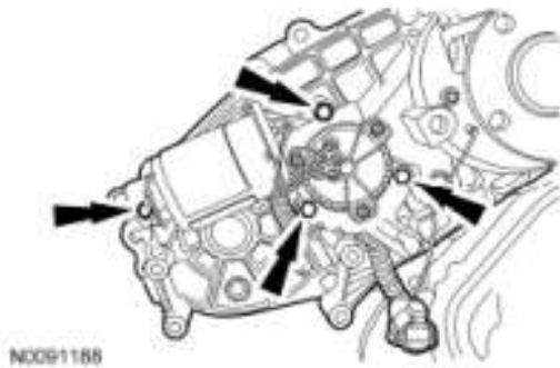
Fig. 103: Locating Shift Motor Bracket Bolt And Shift Motor Bolts Courtesy of FORD MOTOR CO.
