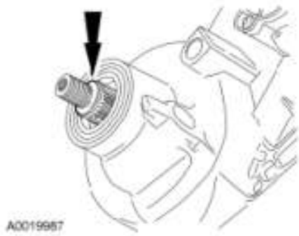
Fig. 18: Locating Oil Seal On Rear Output Shaft Courtesy of FORD MOTOR CO.
