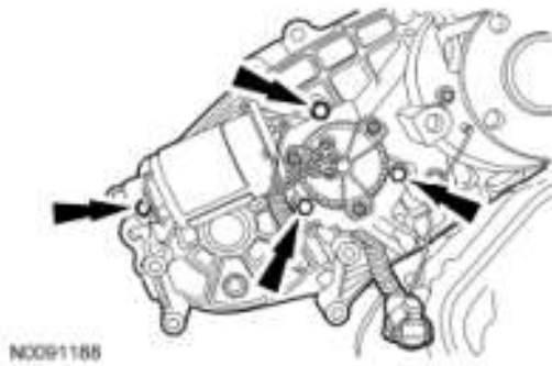
Fig. 21: Locating Shift Motor Bracket Bolt And Shift Motor Bolts Courtesy of FORD MOTOR CO.
