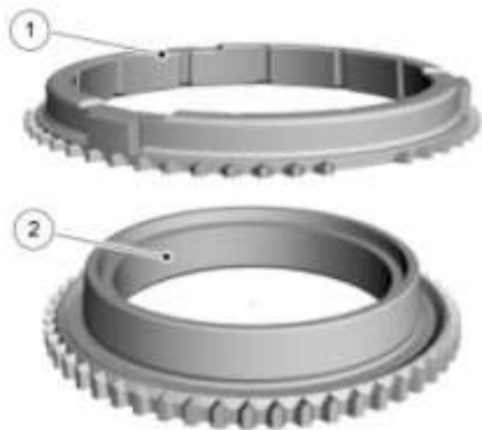
Fig. 16: Identifying Synchronizer Rings For Single Synchronization In 5th/6th/Reverse Gear Courtesy of FORD MOTOR CO.
