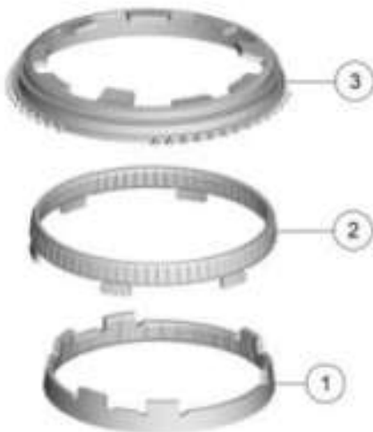
Fig. 14: Identifying Synchronizer Ring For Triple Synchronization In 1st/2nd Gear Courtesy of FORD MOTOR CO.
