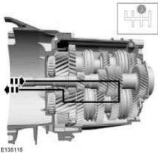
Fig. 9: Power Transmission Route In 3rd Gear Courtesy of FORD MOTOR CO.
