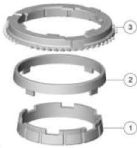
Fig. 15: Identifying Synchronizer Rings For 3rd/4th Gear Double Synchronization Courtesy of FORD MOTOR CO.
