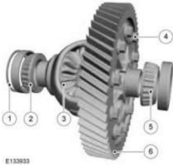
Fig. 6: Identifying Differential Related Components Courtesy of FORD MOTOR CO.
