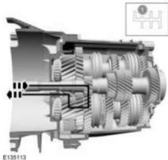
Fig. 7: Power Transmission Route In 1st Gear
