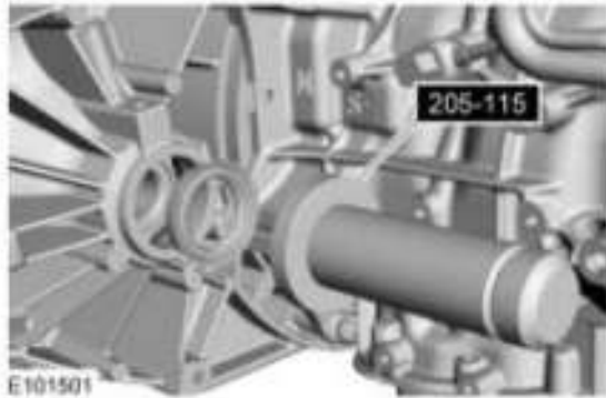
Fig. 34: Installing Drive Pinion Seal Courtesy of FORD MOTOR CO.
