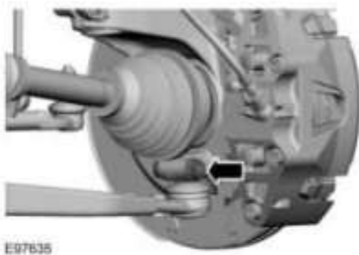
Fig. 77: Locating Lower Control Arm Bolts And Nuts Courtesy of FORD MOTOR CO.
