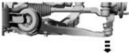
Fig. 77: Locating Lower Control Arm Bolts And Nuts Courtesy of FORD MOTOR CO.
