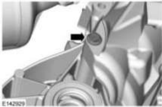
Fig. 90: Locating Transmission Mounting Bolt Courtesy of FORD MOTOR CO.
