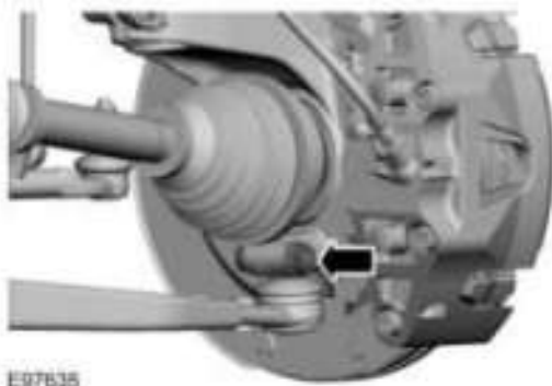
Fig. 107: Locating Lower Control Arm Bolts And Nuts Courtesy of FORD MOTOR CO.
