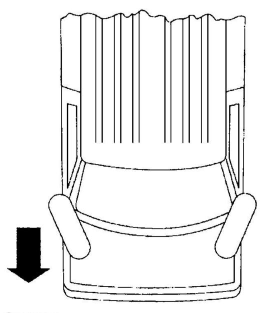
Fig. 3: Identifying Positive Toe (Toe In) Courtesy of FORD MOTOR CO.
