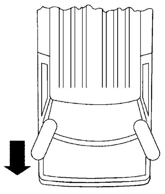
Fig. 4: Identifying Negative Toe (Toe Out) Courtesy of FORD MOTOR CO.
