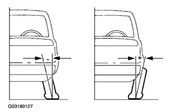
Fig. 1: Identifying Negative And Positive Camber Courtesy of FORD MOTOR CO.
