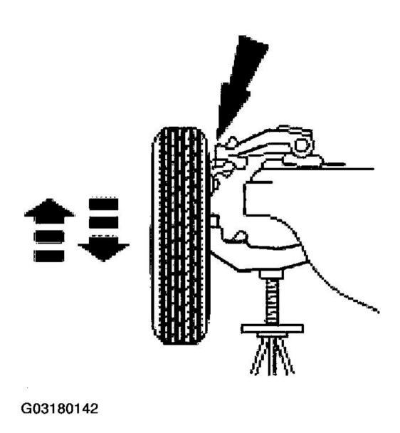
Fig. 16: Inspecting Upper Ball Joint Courtesy of FORD MOTOR CO.
